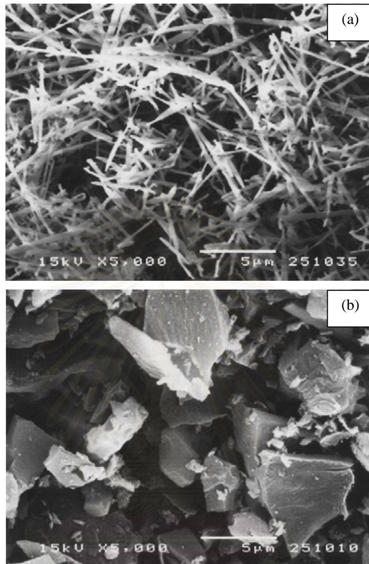
**Figure 4.4** SEM micrographs of product obtained from the carbothermal reduction and nitridation of RHA without hydrogen pretreatment; (a) Top portion, (b) Bottom portion
