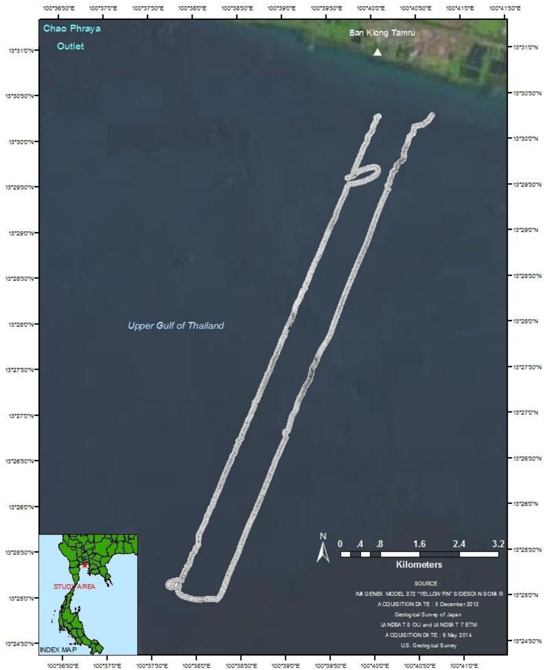
Figure 25 Sonograph of Ban Klong Tamru survey line. Sonograph data is derived from Geological Survey of Japan (2012).
