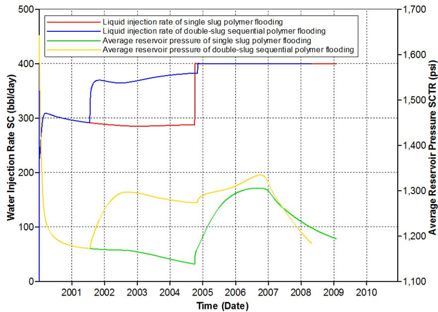
Figure 5.41 Actual injection rates and average reservoir pressures as a function of time of single-slug and double-slug sequential polymer flooding for residual resistance factor of 1.5
