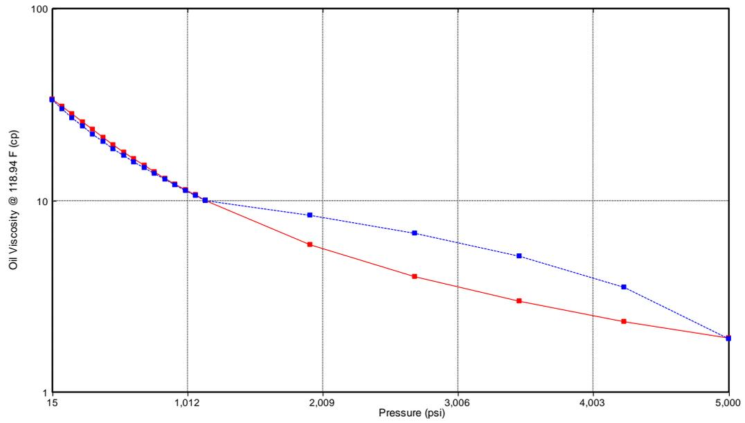
Figure 4.5 Oil viscosity ( $\mu_o$ ) as a function of pressure
