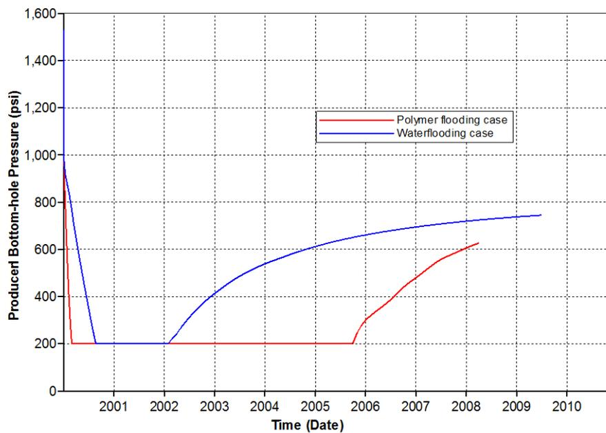
Figure 5.8 Comparison of bottomhole pressure of production well between polymer flooding and waterflooding
