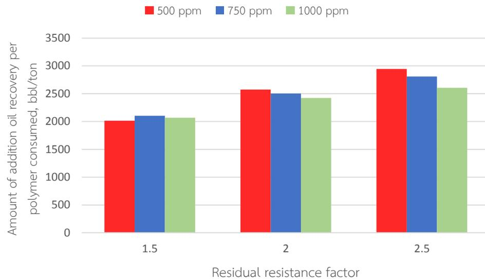
Figure 5.32 Summary of oil recovery factors obtained residual resistance factors of 1.5, 2.0 and 2.5 with different polymer concentrations
