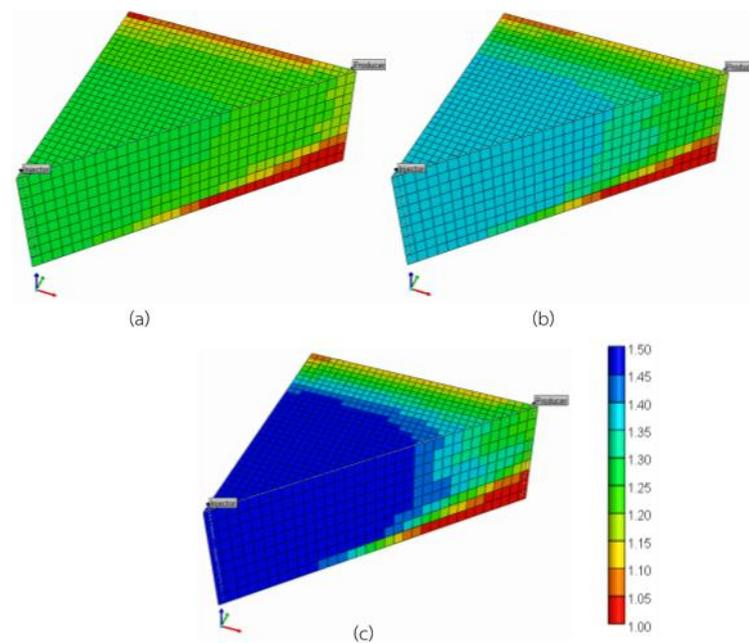
Figure 5.27 Residual resistance factor profile at the end of production (a) polymer concentration of 500 ppm, (b) polymer concentration of 750 ppm and (c) polymer concentration of 1,000 ppm
