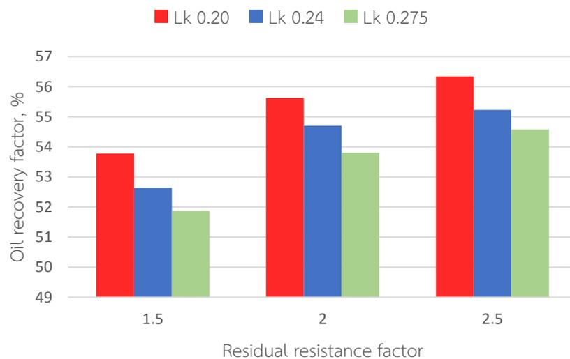
Figure 5.67 Comparison of oil recovery factor among different heterogeneities of single-slug polymer base case for polymer solutions with different residual resistance factors
