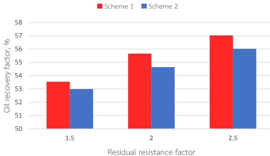
*Figure 5.55 Comparison of oil recovery factor between low concentration and high concentration contrast in sequential polymer flooding for polymer solutions with different residual resistance factors*
