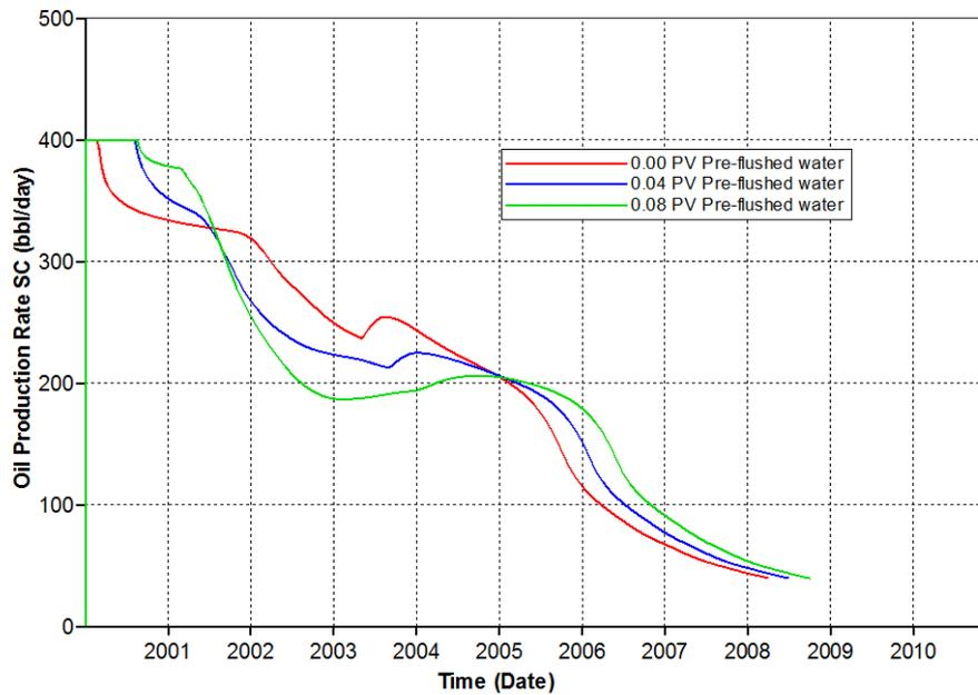
Figure 5.17 Oil production rates of different pre-flushed water slug sizes for polymer concentration of 750 ppm
