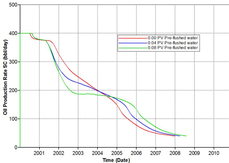
Figure 5.16 Oil production rates of different pre-flushed water slug sizes for polymer concentration of 500 ppm
