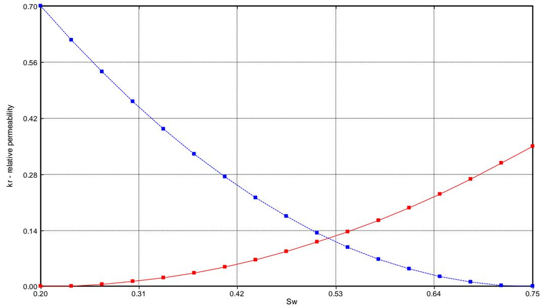
Figure 4.10 Relative permeability of oil-water system as a function of water saturation
