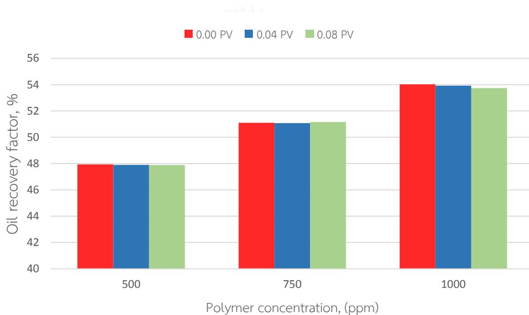
*Figure 5.19 Summary of oil recovery factors obtained from polymer flooding with concentration of 500, 750 and 1,000 ppm with different pre-flushed water slug sizes*
