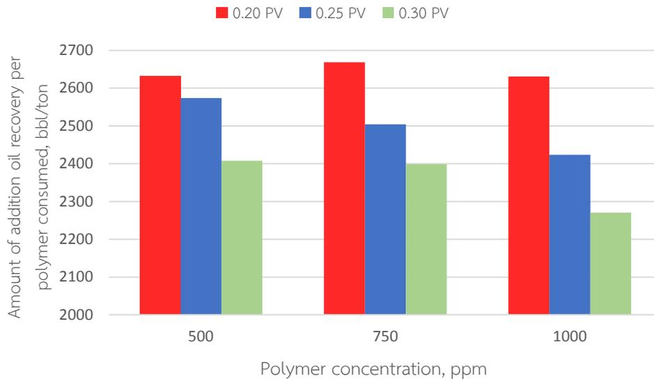
*Figure 5.37 Summary of additional oil recovered per polymer consumed of polymer flooding with polymer concentration of 500, 750 and 1,000 ppm at different polymer slug sizes*
