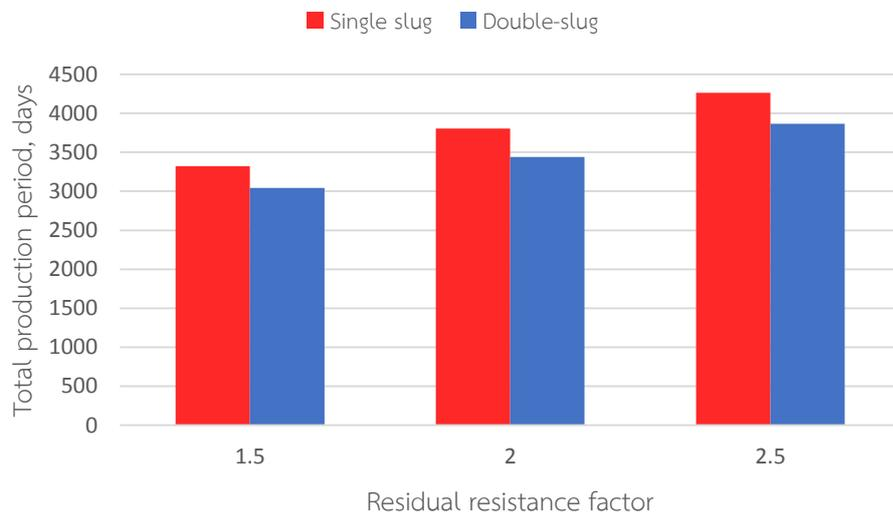
Figure 5.50 Comparison of total production period between single-slug and double-slug sequential polymer flooding for polymer solutions with different residual resistance factors
