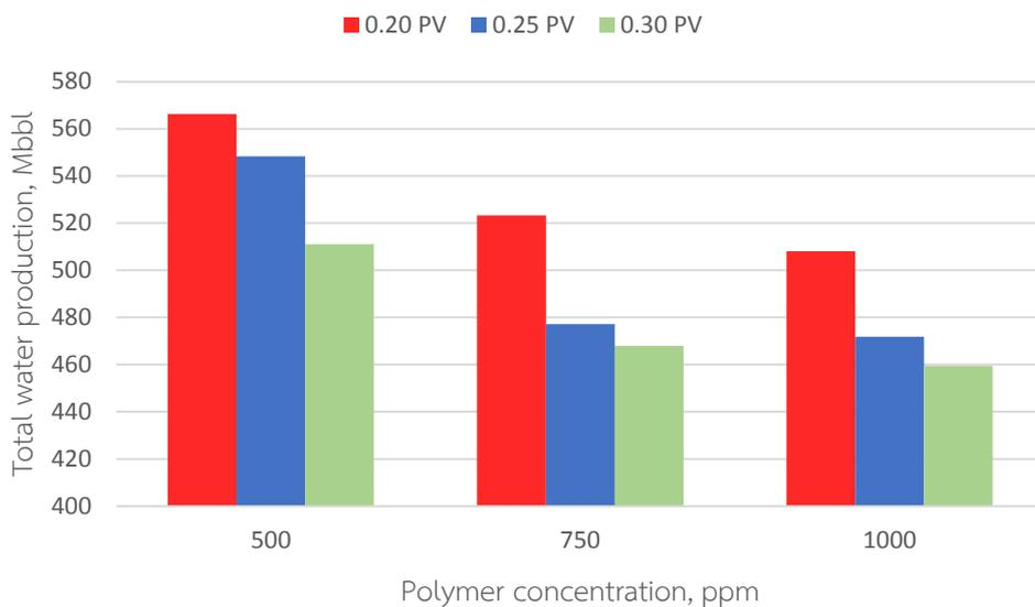
Figure 5.35 Summary of total water productions of polymer flooding with polymer concentration of 500, 750 and 1,000 ppm at different polymer slug sizes
