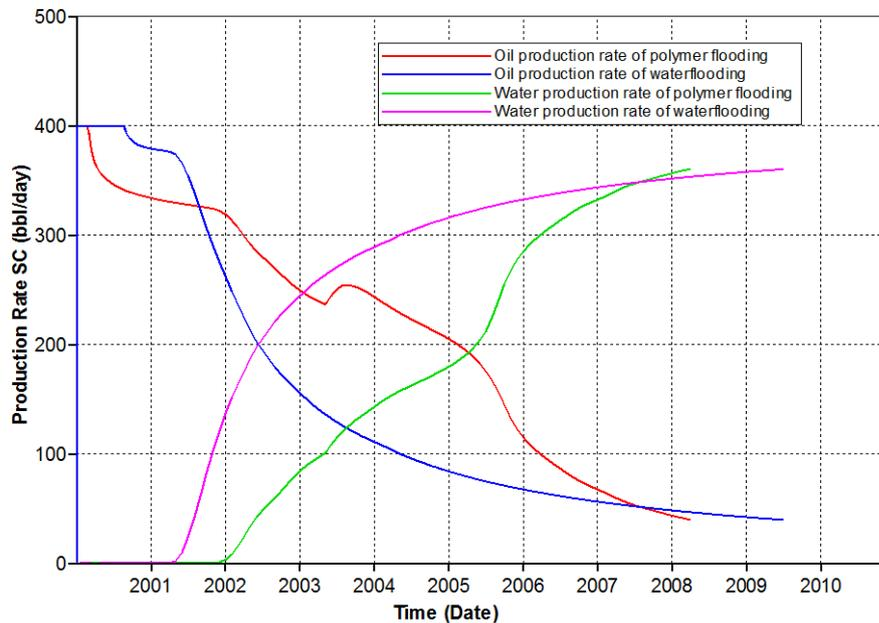
Figure 5.7 Comparison of oil and water production rates between polymer flooding and waterflooding
