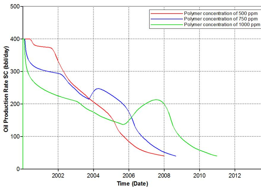
Figure 5.30 Oil production rates of different polymer concentrations for polymer solution with residual resistance factor of 2.5
