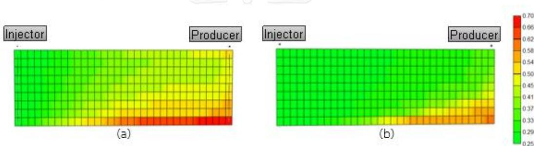
Figure 5.12 Oil saturation profile from side view of a) waterflooding case and b) polymer flooding case at the end of production
