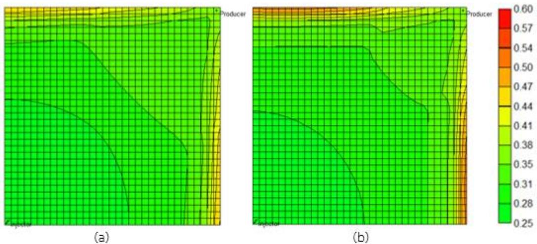
Figure 5.47 Oil saturation profile of high permeability layer (top layer) of a) single-slug polymer flooding and b) double-slug sequential polymer
