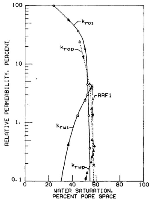
Figure 3.6 Relative permeability to oil and to water before and after contact with commercial polymer solution (Dow pusher 1000<sup>TM</sup>) [13]
