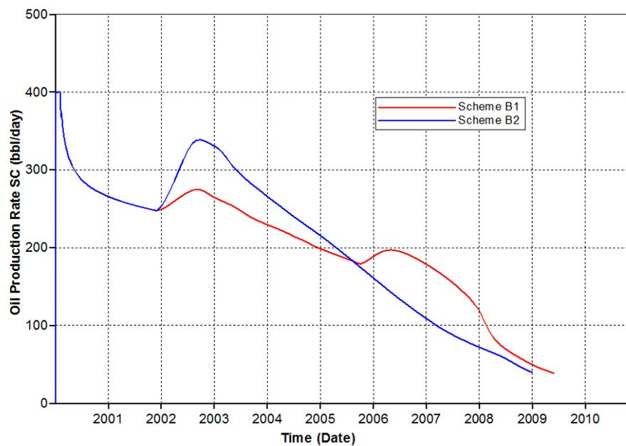
Figure 5.53 Oil production rates of double-slug sequential polymer flooding with different second slug concentrations for polymer solution with residual resistance factor of 2.0
