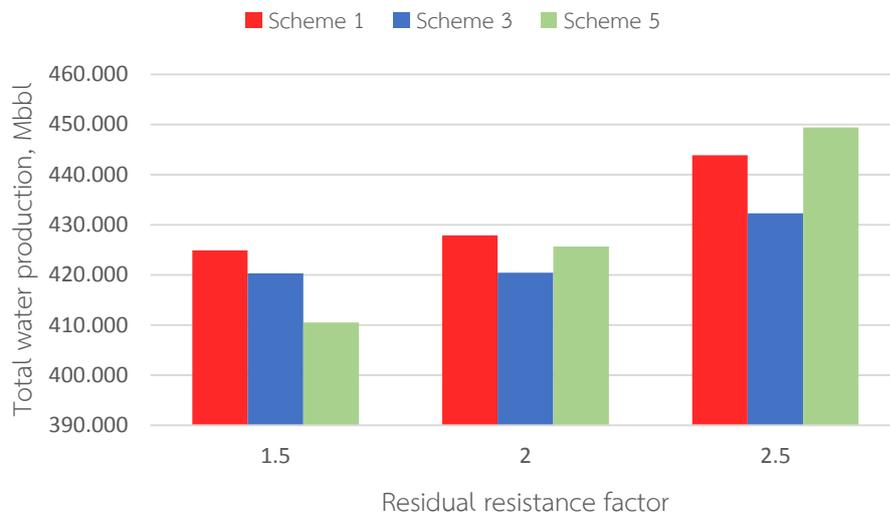
*Figure 5.66 Comparison of total water production among different sizes of first polymer slug with second slug size of 750 ppm polymer concentration for polymer solutions with different residual resistance factors*
