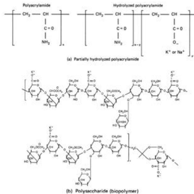
Figure 3.1 Molecular structure of a) synthetic polymer (HPAM) and b) Xanthan biopolymer (Polysaccharide) [10]
