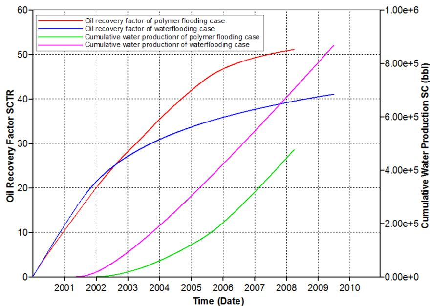
Figure 5.10 Comparison of oil recovery factor between polymer flooding case and waterflooding case as a function of time
