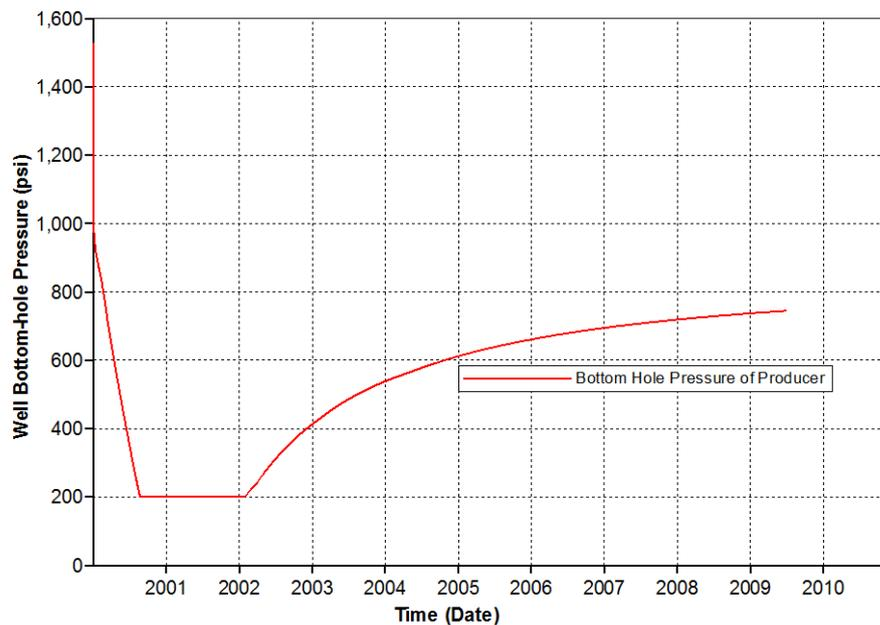
Figure 5.3 Bottomhole pressure of production well of waterflooding case as a function of time
