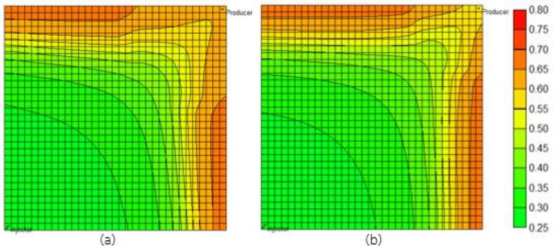
Figure 5.48 Oil saturation profile of low permeability layer (8<sup>th</sup> layer) of a) single-slug polymer flooding and b) double-slug sequential polymer
