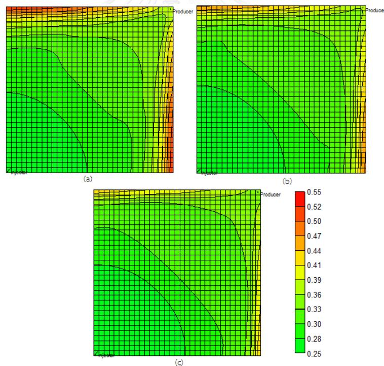
Figure 5.36 Oil saturation profile in the uppermost layer at the end of production in case of polymer concentration of 1,000 ppm (a) polymer solution slug 0.2 PV (b) polymer solution slug 0.25 PV and (c) polymer solution slug 0.3 PV
