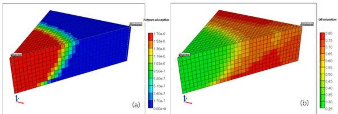
Figure 5.9 a) Polymer adsorption profile and b) oil saturation profile of polymer flooding case at the day of water breakthrough
