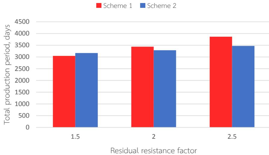
Figure 5.56 Comparison of total production period between low concentration and high concentration contrast in sequential polymer flooding for polymer solutions with different residual resistance factors
