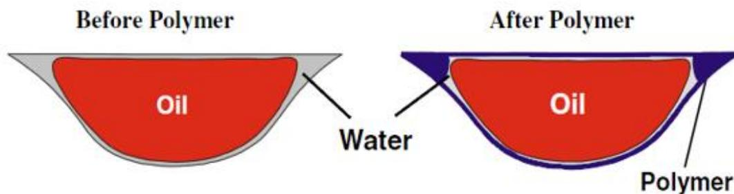
Figure 3.4 Illustration of permeability reduction mechanism [2]
