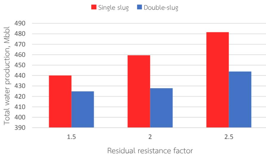
Figure 5.51 Comparison of total water production between single-slug and double-slug sequential polymer flooding for polymer solutions with different residual resistance factors
