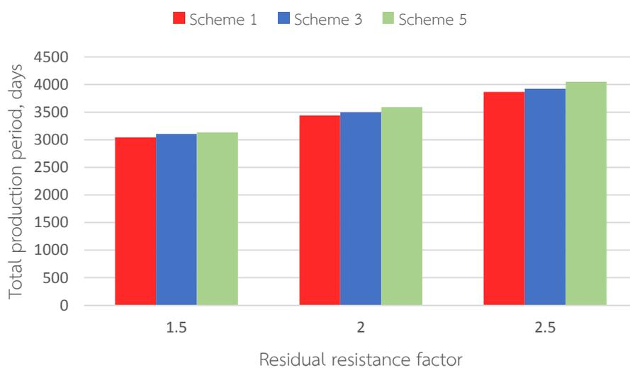
*Figure 5.65 Comparison of total production period among different sizes of first polymer slug with second slug size of 750 ppm polymer concentration for polymer solutions with different residual resistance factors*
