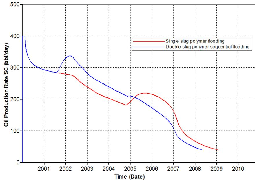
Figure 5.44 Oil production rates of single-slug and double-slug sequential polymer flooding for polymer solution with residual resistance factor of 1.5
