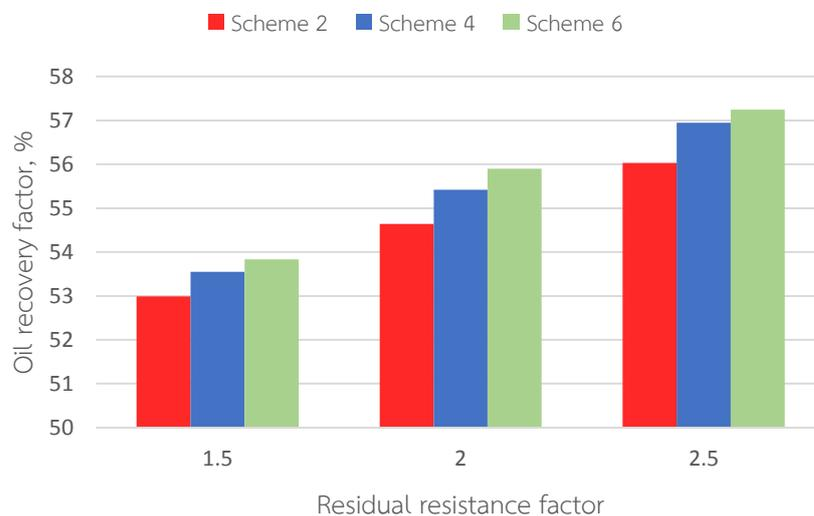
Figure 5.61 Comparison of oil recovery factor among different sizes of first polymer slug with second slug size of 500 ppm polymer concentration for polymer solutions with different residual resistance factors
