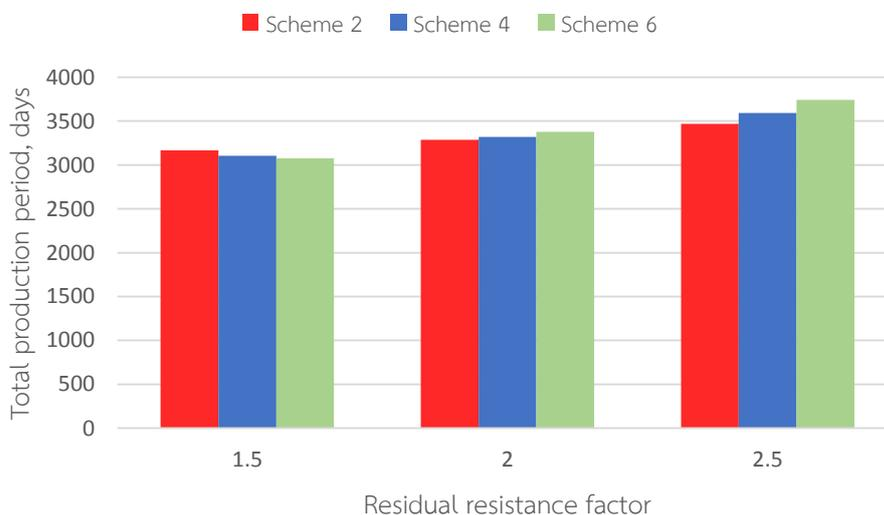
Figure 5.62 Comparison of total production time among different sizes of first polymer slug with second slug size of 500 ppm polymer concentration for polymer solutions with different residual resistance factors
