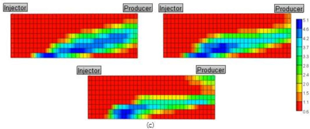
Figure 5.73 Water viscosity profile from side view at the end of production in case of double-slug sequential polymer flooding base case with residual resistance factor 1.5 (a)  $L_k = 0.2$  (b)  $L_k = 0.24$  and (c)  $L_k = 0.275$
