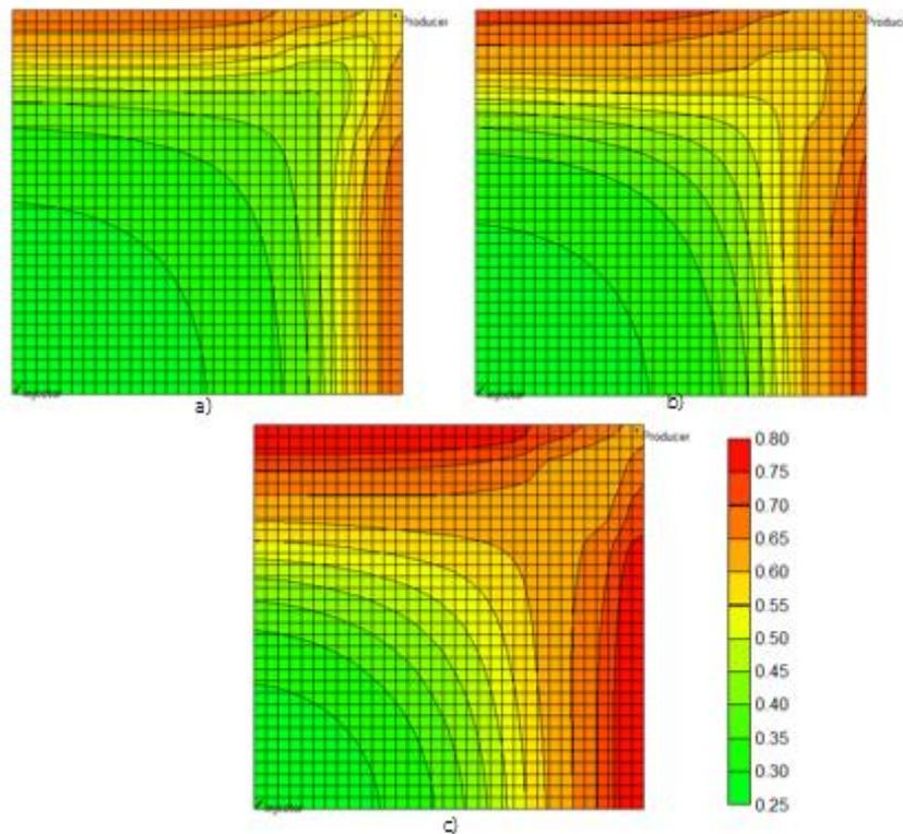
Figure 5.76 Oil saturation profile of low permeability zone (8th layer) at the end of production of triple-slug sequential polymer with residual resistance factor of 1.5 with different degree of heterogeneity (a)  $L_k = 0.2$  (b)  $L_k = 0.24$  and (c)  $L_k = 0.275$
