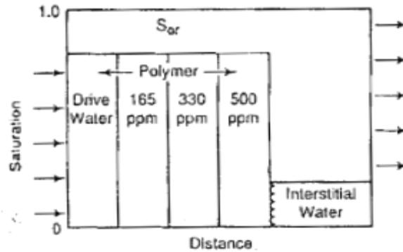
Figure 3.2 Injection schedule for a continuous polymer flooding [12]
