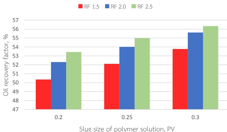
Figure 5.38 Summary of oil recovery factors of polymer flooding with polymer slug size of 0.2, 0.25 and 0.3 PV at different residual resistance factors
