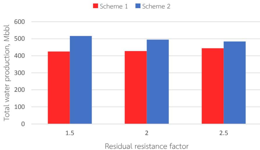
Figure 5.57 Comparison of total water production between low concentration and high concentration contrast in sequential polymer flooding for polymer solutions with different residual resistance factors
