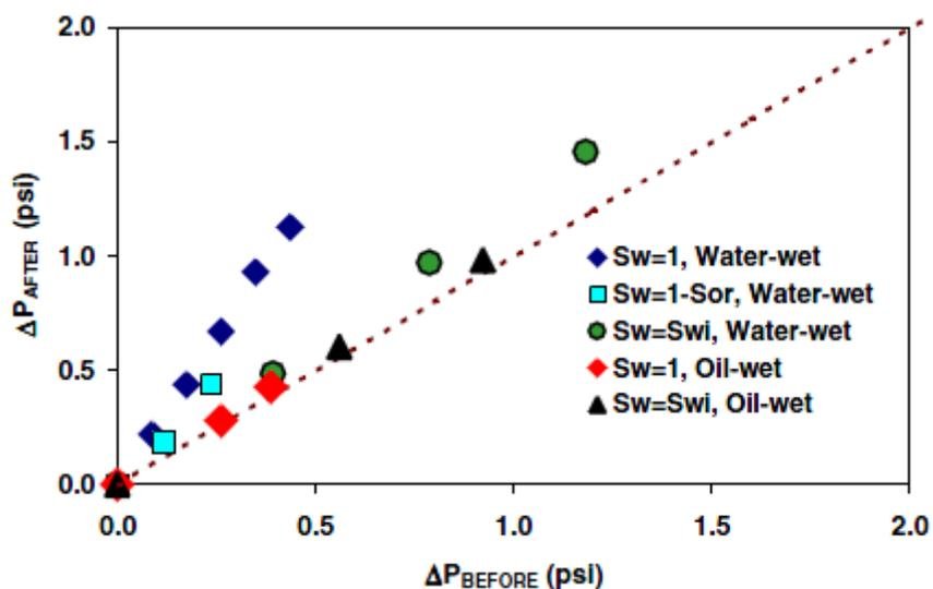
Figure 3.5 Pressure drop from injection process before and after polymer injection of water-wet and oil-wet condition [2]
