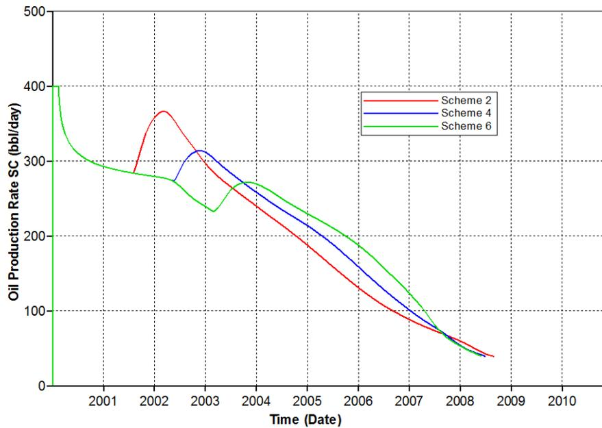
Figure 5.58 Oil production rates of double-slug sequential polymer flooding with different first polymer slug sizes and second slug with concentration of 500 ppm for polymer solution with residual resistance factor of 1.5
