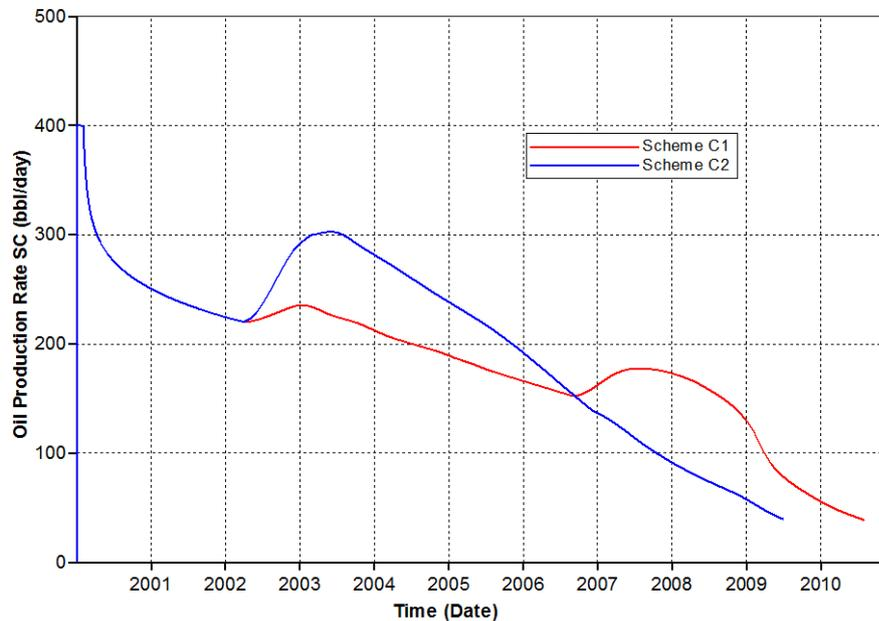
Figure 5.54 Oil production rates of double-slug sequential polymer flooding with different second slug concentrations for polymer solution with residual resistance factor of 2.5
