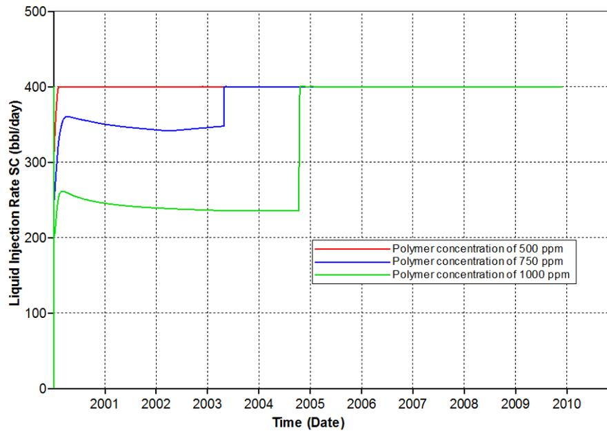
Figure 5.25 Actual liquid injection rates of different polymer concentrations for polymer solution with residual resistance factor of 2.0
