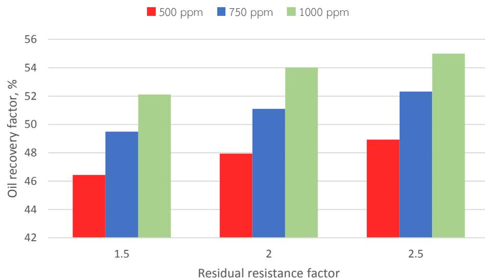
Figure 5.31 Summary of oil recovery factors obtained residual resistance factors of 1.5, 2.0 and 2.5 with different polymer concentrations
