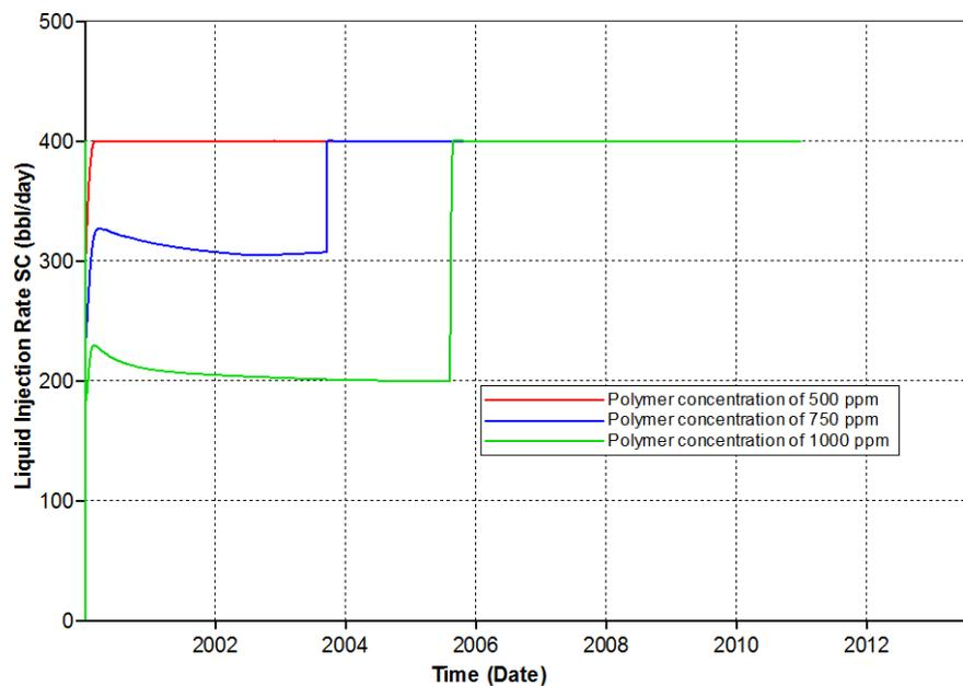
Figure 5.26 Actual liquid injection rates of different polymer concentrations for polymer solution with residual resistance factor of 2.5
