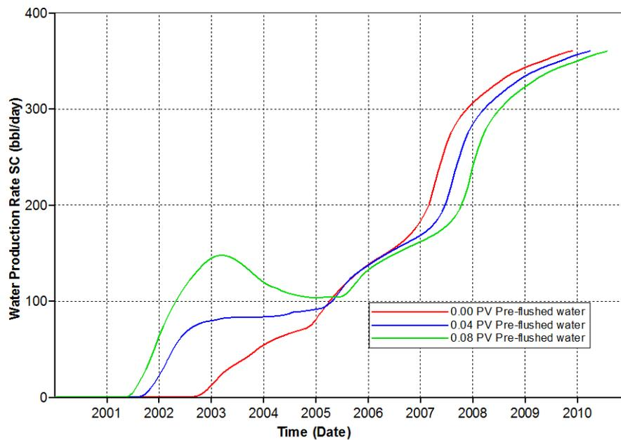
Figure 5.22 Water production rates of different pre-flushed water slug sizes for polymer concentration of 1,000 ppm
