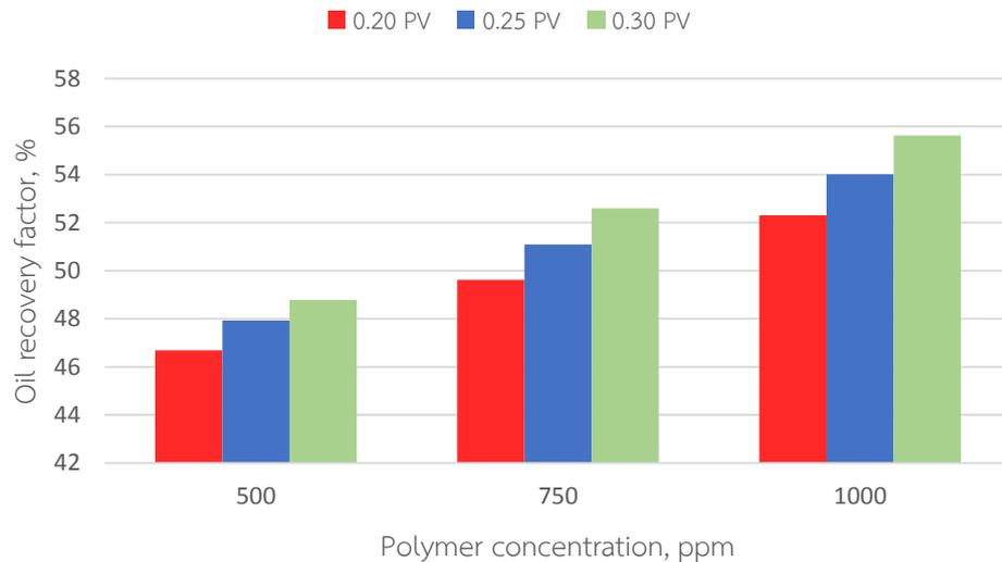
Figure 5.34 Summary of oil recovery factors of polymer flooding with polymer concentration of 500, 750 and 1,000 ppm at different polymer slug sizes
