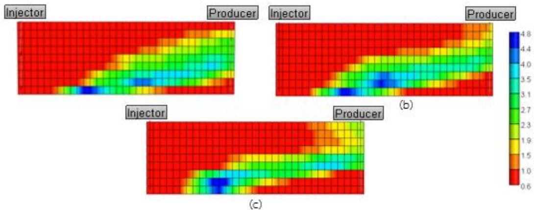
Figure 5.74 Water viscosity profile from side view at the end of production in case of triple-slug sequential polymer flooding base case with residual resistance factor 1.5 (a)  $L_k = 0.2$  (b)  $L_k = 0.24$  and (c)  $L_k = 0.275$
