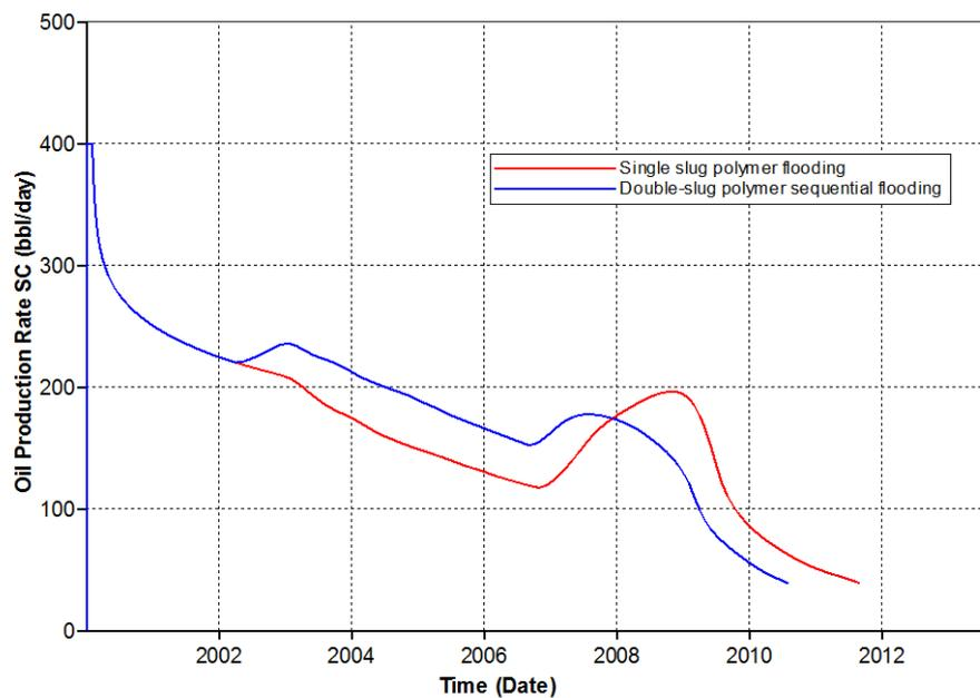
Figure 5.46 Oil production rates of single-slug and double-slug sequential polymer flooding for polymer solution with residual resistance factor of 2.5
