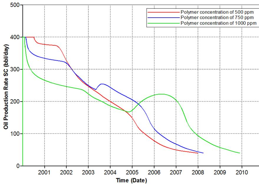
Figure 5.29 Oil production rates of different polymer concentrations for polymer solution with residual resistance factor of 2.0
