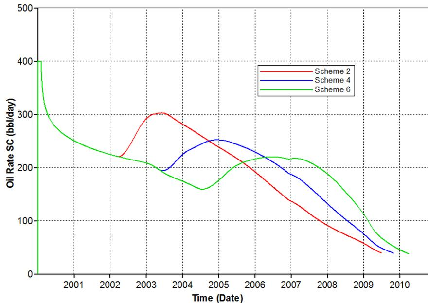
Figure 5.60 Oil production rates of double-slug sequential polymer flooding with different first polymer slug sizes and second slug with concentration of 500 ppm for polymer solution with residual resistance factor of 2.5
