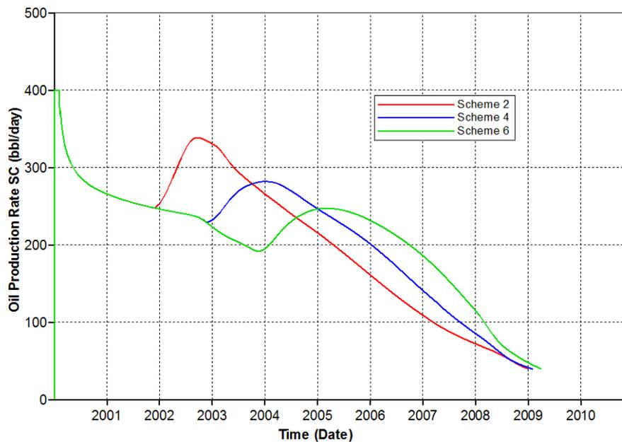
Figure 5.59 Oil production rates of double-slug sequential polymer flooding with different first polymer slug sizes and second slug with concentration of 500 ppm for polymer solution with residual resistance factor of 2.0
