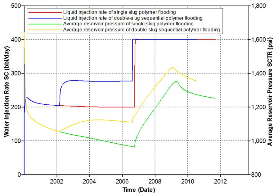
Figure 5.43 Actual injection rates and average reservoir pressures as a function of time of single-slug and double-slug sequential polymer flooding for residual resistance factor of 2.5
