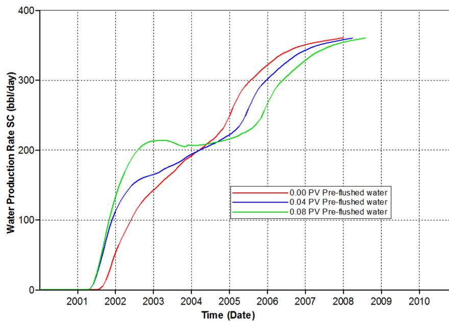
Figure 5.20 Water production rates of different pre-flushed water slug sizes for polymer concentration of 500 ppm
