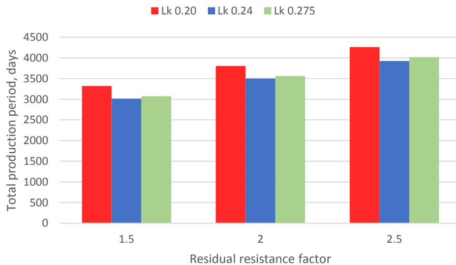
Figure 5.71 Comparison of total production period among different heterogeneity of single-slug polymer base case for polymer solutions with different residual resistance factors
