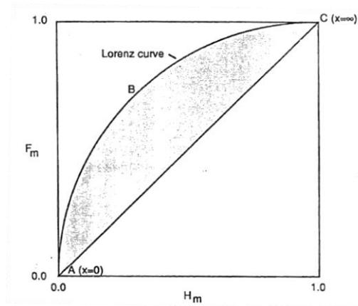
Figure 3.9 Flow capacity distribution representing Lorenz curve [14]
