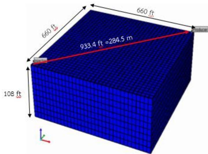
Figure 4.1 Dimension of reservoir model and location of injector and producer
