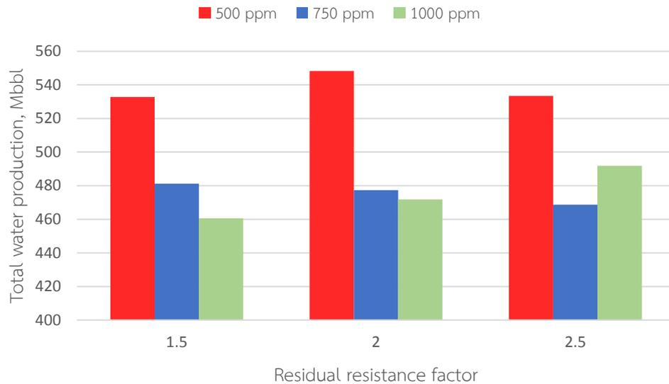
*Figure 5.33 Summary of total water production of polymer flooding with maximum resistance factor of 1.5, 2.0 and 2.5 at different polymer concentration*
