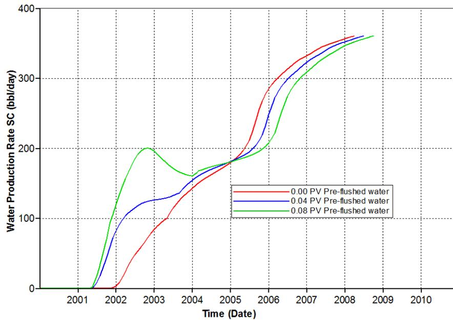
Figure 5.21 Water production rates of different pre-flushed water slug sizes for polymer concentration of 750 ppm
