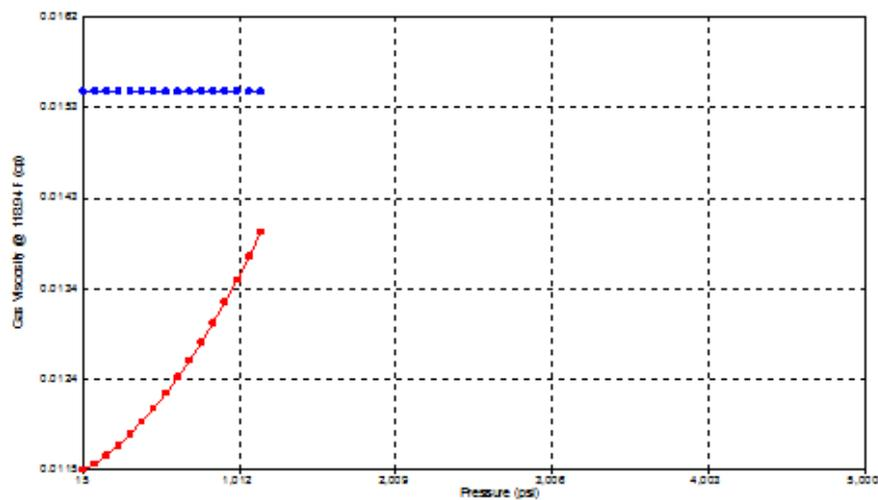
Figure 4.9 Gas viscosity ( $\mu_g$ ) as a function of pressure
