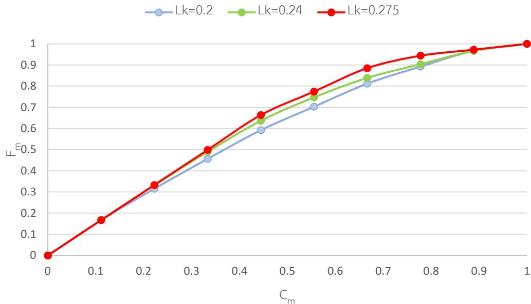
Figure 4.3 Summary of flow capacity distribution for reservoir models with different Lorenz coefficients
