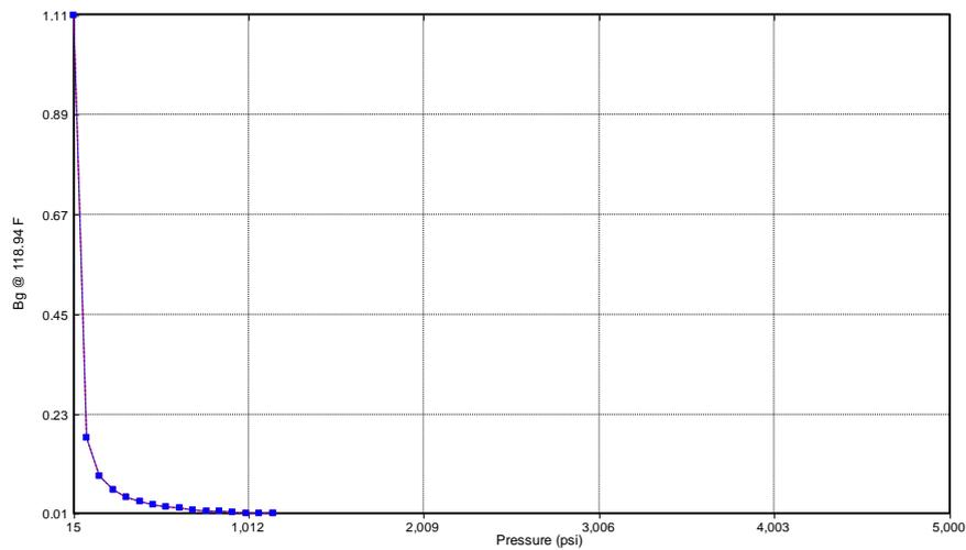
Figure 4.8 Formation volume factor of dry gas ( $B_g$ ) as a function of pressure
