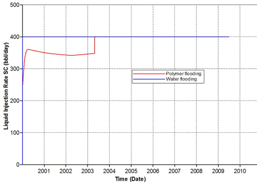
Figure 5.6 Comparison of liquid injection rate between polymer flooding base case and waterflooding
