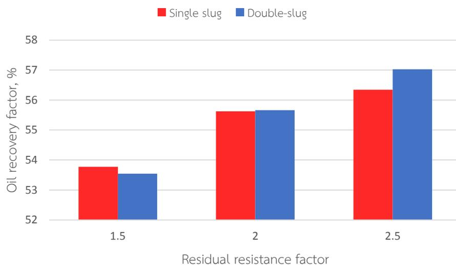
*Figure 5.49 Comparison of oil recovery factor between single-slug and double-slug sequential polymer flooding for polymer solutions with different residual resistance factors*
