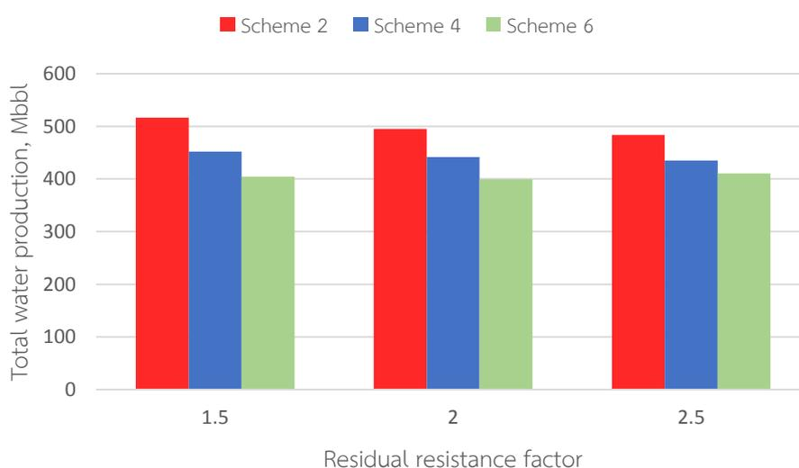
Figure 5.63 Summary of total water production of double-slug sequential polymer flooding with different size of first slug with second slug concentration of 500 ppm for different of residual resistance factor
