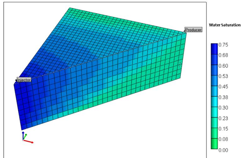
Figure 5.5 Water saturation profile at period of water breakthrough (top layer) in waterflooding case.
