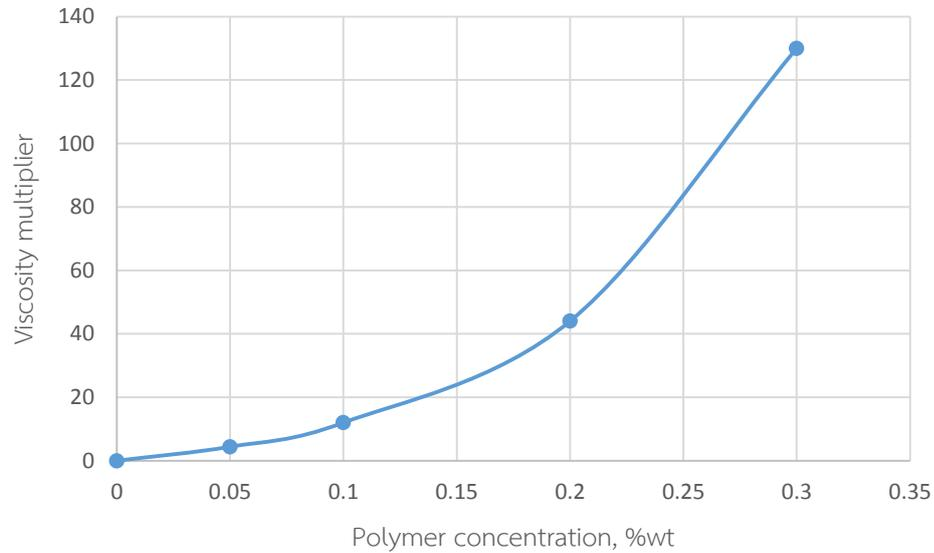
Figure 4.12 Relation of viscosity multiplier as a function of polymer concentration
