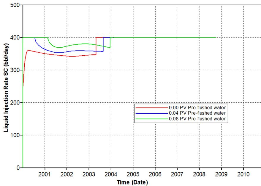
Figure 5.14 Actual liquid injection rates of different pre-flushed water slug sizes for polymer concentration of 750 ppm
