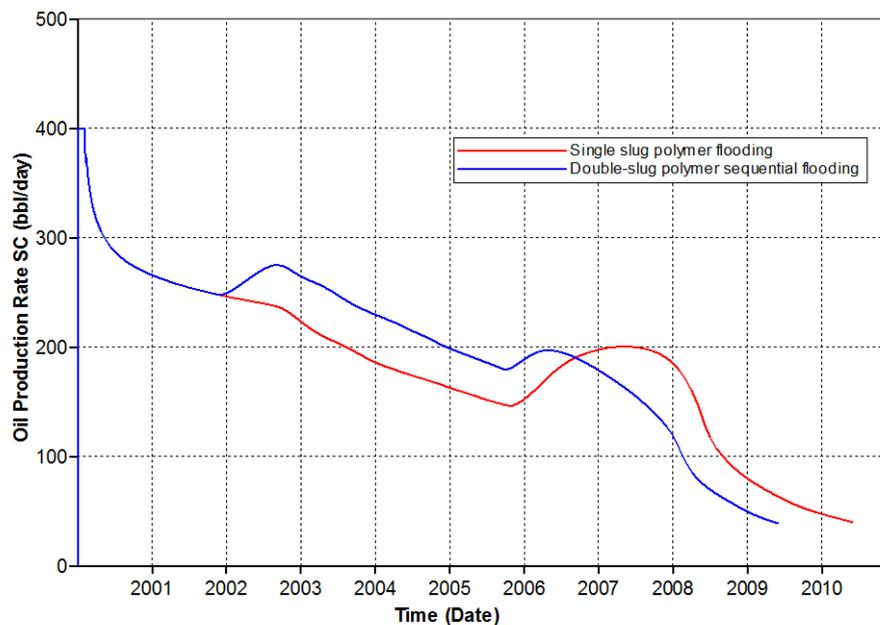
Figure 5.45 Oil production rates of single-slug and double-slug sequential polymer flooding for polymer solution with residual resistance factor of 2.0
