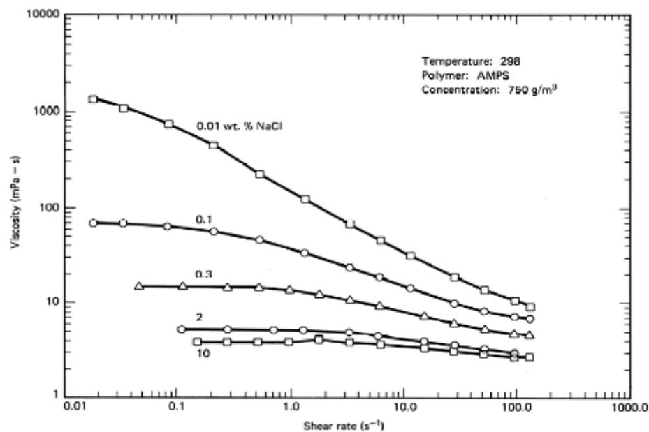
Figure 3.3 Viscosity of polymer solutions with different salinities as a function of shear rate [10]
