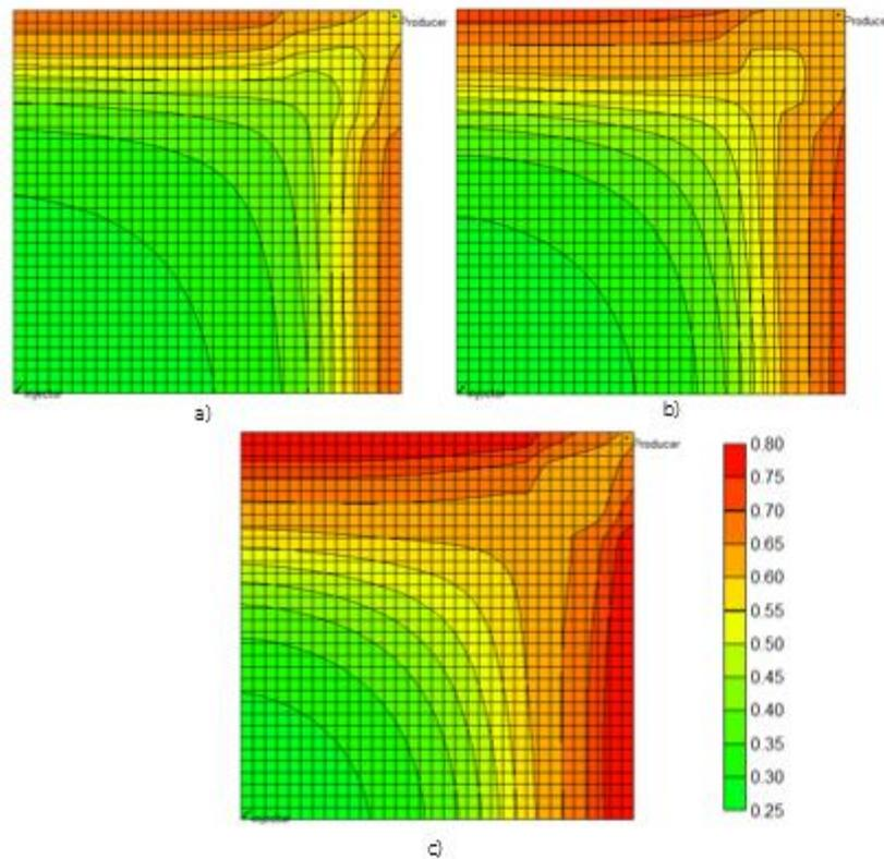
Figure 5.75 Oil saturation profile of low permeability zone (8<sup>th</sup> layer) at the end of production of double-slug sequential polymer with residual resistance factor of 1.5 with different degree of heterogeneity (a)  $L_k = 0.2$  (b)  $L_k = 0.24$  and (c)  $L_k = 0.275$
