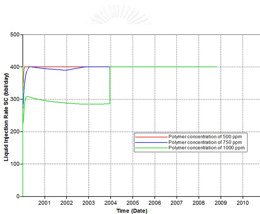
Figure 5.24 Actual liquid injection rates of different polymer concentrations for polymer solution with residual resistance factor of 1.5
