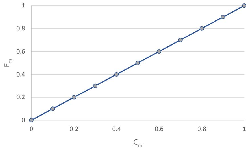
Figure 4.2 Flow capacity distribution for homogeneous reservoir
