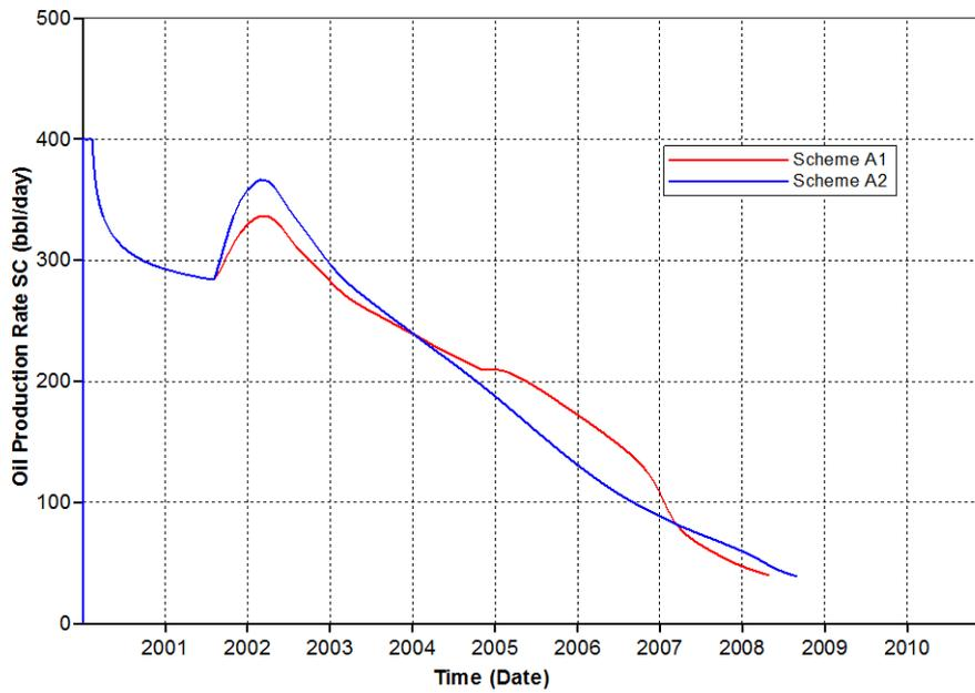
Figure 5.52 Oil production rates of double-slug sequential polymer flooding with different second slug concentrations for polymer solution with residual resistance factor of 1.5
