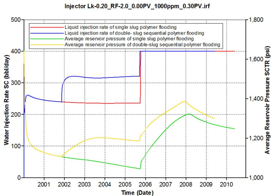
Figure 5.42 Actual injection rates and average reservoir pressures as a function of time of single-slug and double-slug sequential polymer flooding for residual resistance factor of 2.0
