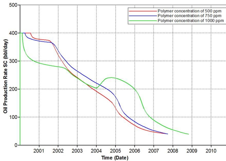
Figure 5.28 Oil production rates of different polymer concentrations for polymer solution with residual resistance factor of 1.5
