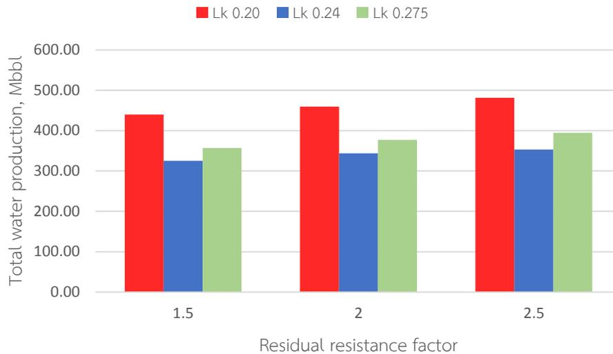
*Figure 5.72 Comparison of total water production among different heterogeneity of single-slug polymer base case for polymer solutions with different residual resistance factors*
