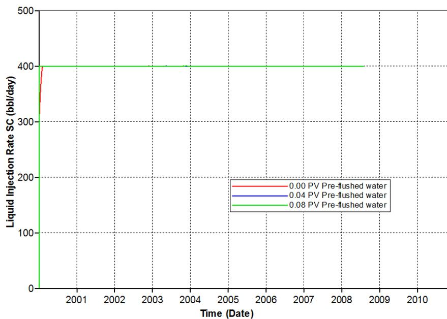
Figure 5.13 Actual liquid injection rates of different pre-flushed water slug sizes for polymer concentration of 500 ppm
