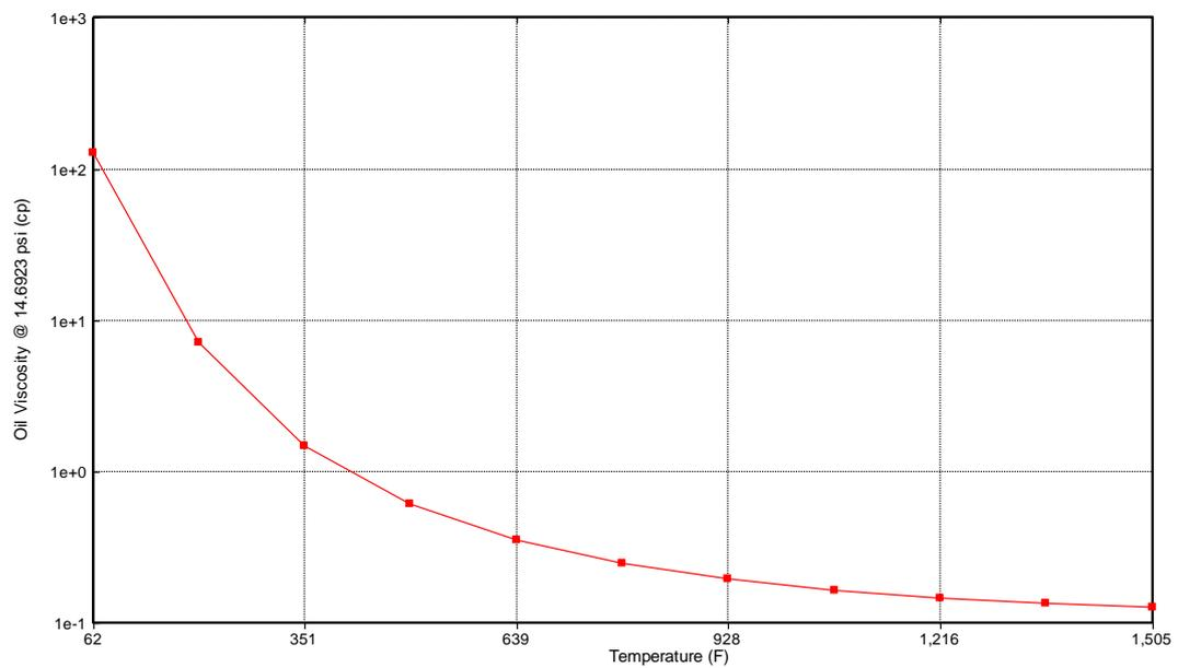
Figure 4.6 Oil viscosity ( $\mu_o$ ) as a function of temperature
