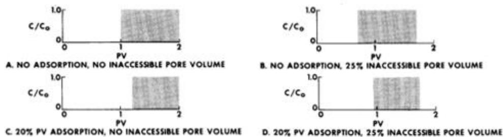
Figure 3.8 Ideal polymer break out curve, polymer bank size = 1.0 PV [14]
