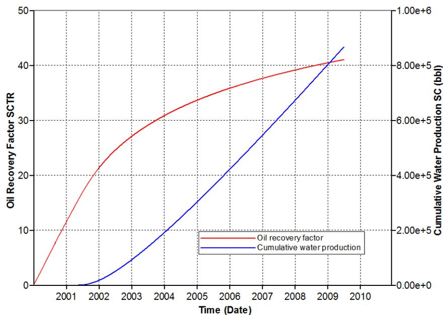
Figure 5.4 Oil recovery factor and cumulative water production of waterflooding case as a function of time
