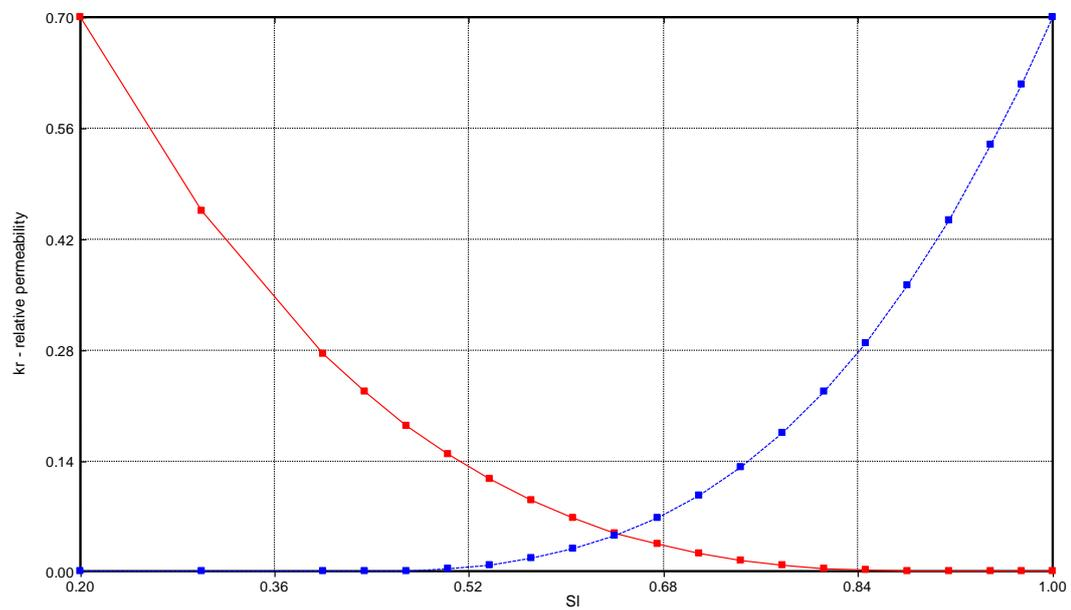
Figure 4.11 Relative permeability of gas-liquid system as a function of liquid saturation
