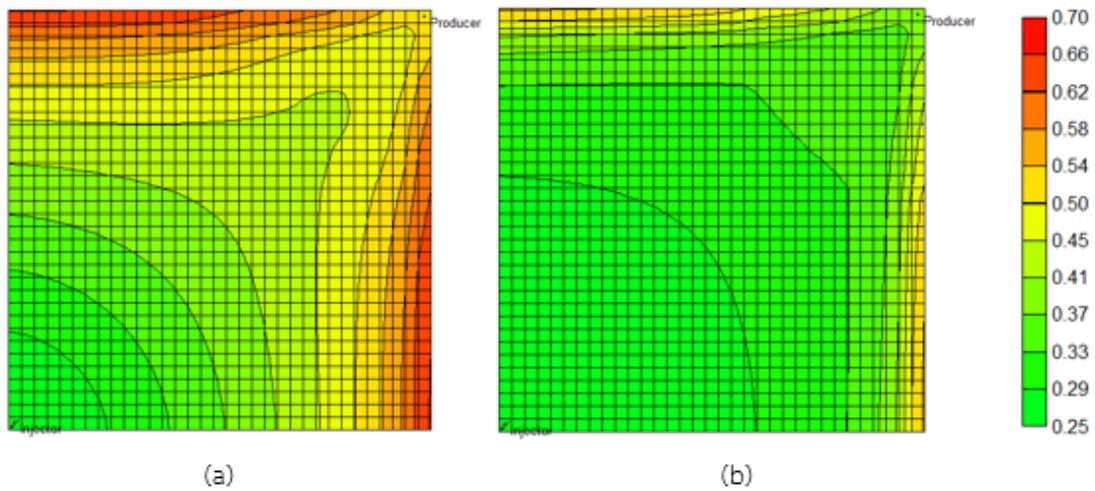
Figure 5.11 Oil saturation profile from top view of a) waterflooding case and b) polymer flooding case at the end of production
