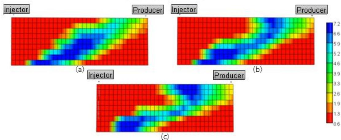
Figure 5.69 Water viscosity profile from side view after 2 year of chasing water injection in case of single-slug polymer flooding base case with residual resistance factor 1.5 (a)  $L_k = 0.2$  (b)  $L_k = 0.24$  and (c)  $L_k = 0.275$
