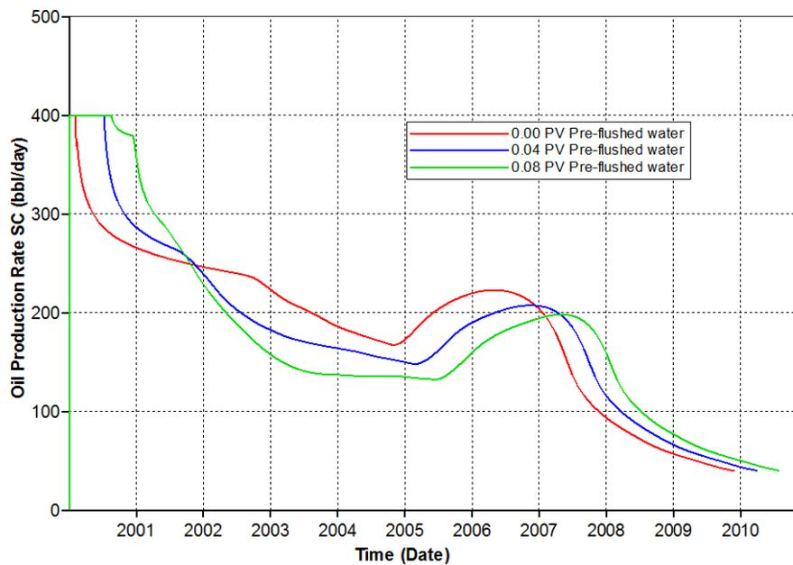
Figure 5.18 Oil production rates of different pre-flushed water slug sizes for polymer concentration of 1,000 ppm
