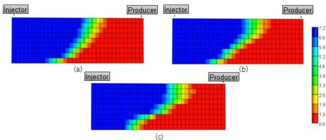
Figure 5.68 Water viscosity profile from side view at the day before inject chasing water in case of single-slug polymer flooding base case with residual resistance factor 1.5 (a)  $L_k = 0.2$  (b)  $L_k = 0.24$  and (c)  $L_k = 0.275$
