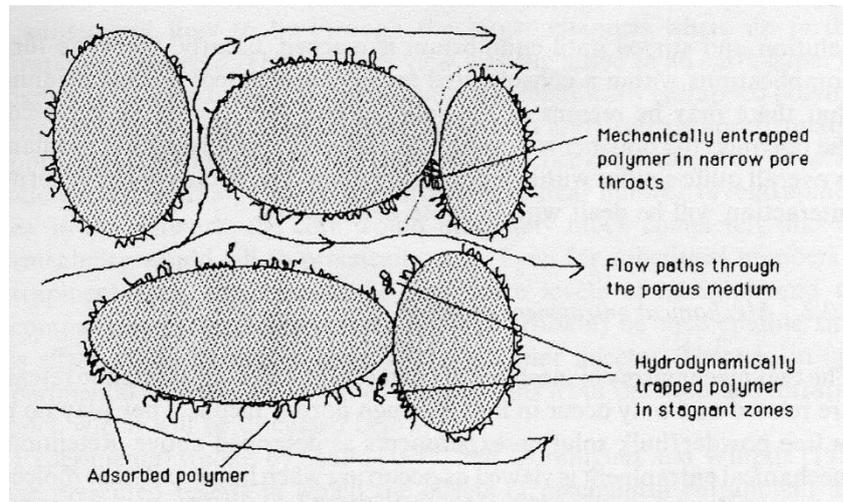
Figure 3.7 Schematic diagram of polymer retention mechanism in porous media [11]
