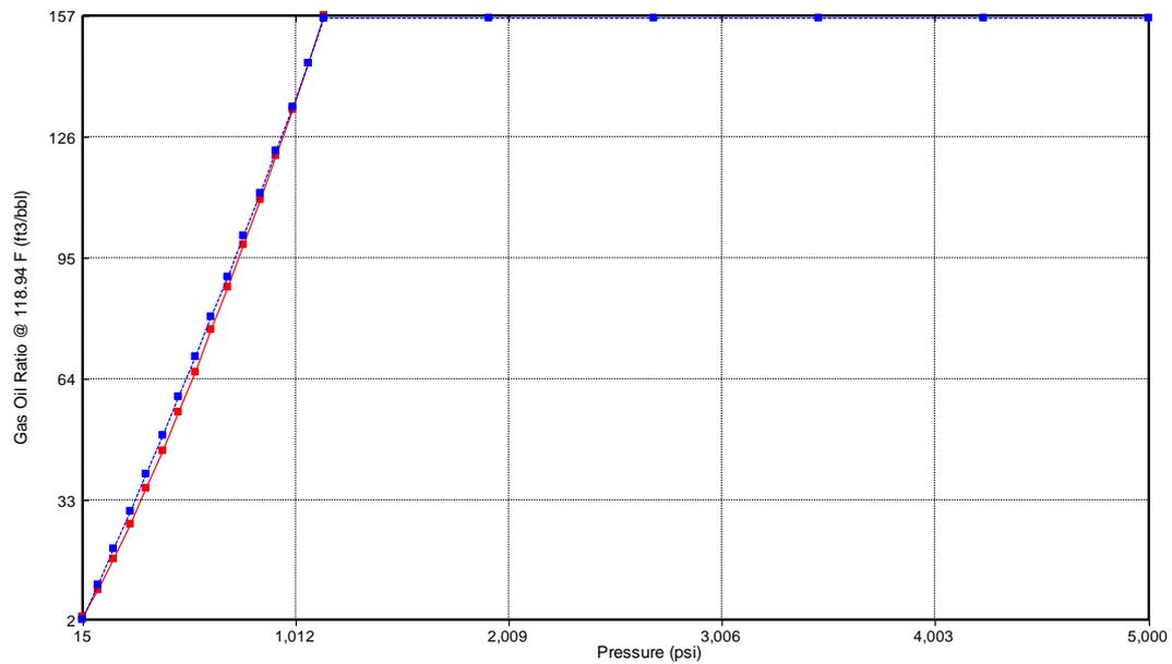
Figure 4.7 Gas/Oil ratio ( $R_s$ ) as a function of pressure
