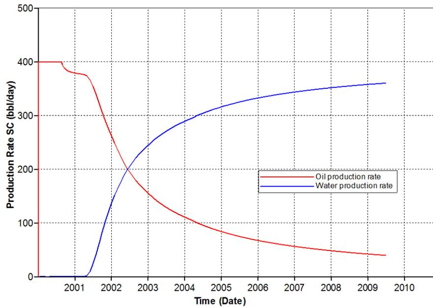
Figure 5.2 Oil and water production rate of waterflooding case as a function of time
