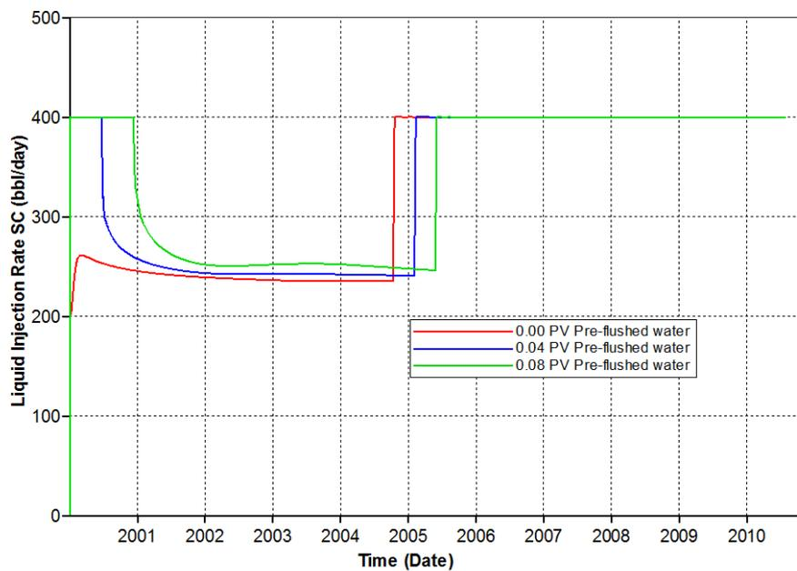
Figure 5.15 Actual liquid injection rates of different pre-flushed water slug sizes for polymer concentration of 1,000 ppm
