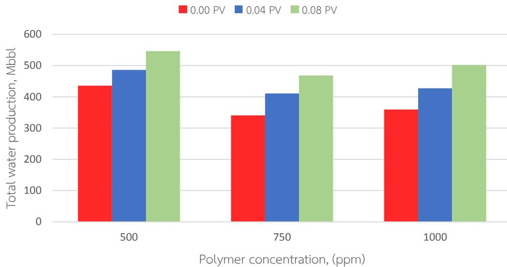
Figure 5.23 Summary of total water production obtained from polymer flooding with concentration of 500, 750 and 1,000 ppm with different pre-flushed water slug sizes
