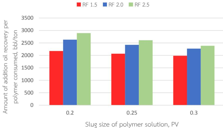
Figure 5.39 Summary of additional oil recovered per polymer consumed of polymer flooding with polymer slug size of 0.2, 0.25 and 0.3 PV at different residual resistance factors
