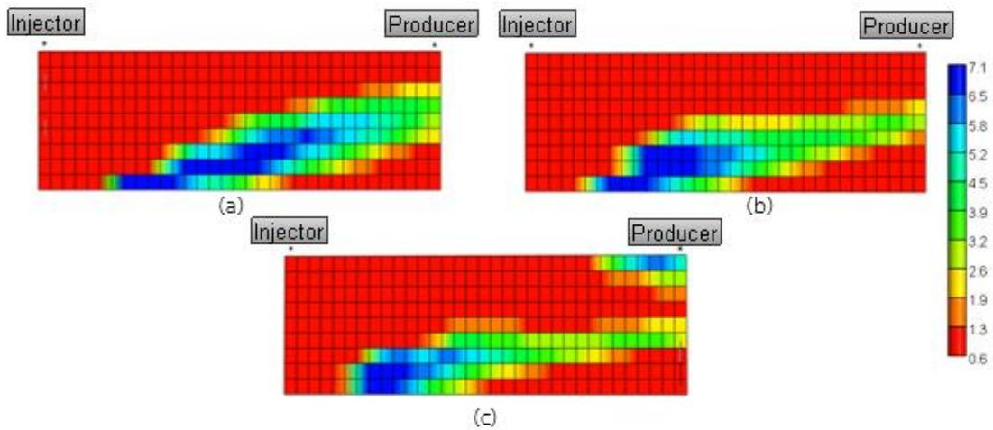
Figure 5.70 Water viscosity profile from side view at the end of production in case of single-slug polymer flooding base case with residual resistance factor 1.5 (a)  $L_k = 0.2$  (b)  $L_k = 0.24$  and (c)  $L_k = 0.275$
