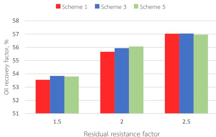
Figure 5.64 Comparison of oil recovery factor among different sizes of first polymer slug with second slug size of 750 ppm polymer concentration for polymer solutions with different residual resistance factors
