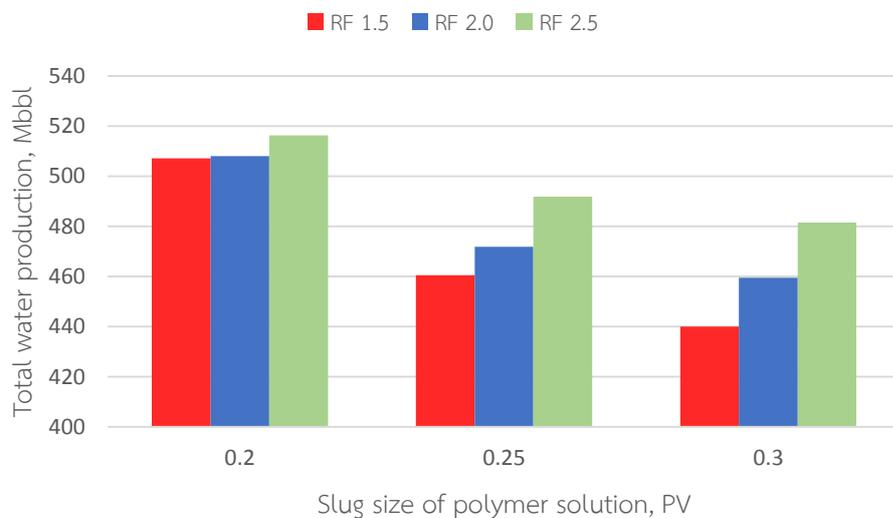
Figure 5.40 Summary of total water production of polymer flooding with polymer solution slug size of 0.2, 0.25, 0.3 PV at different residual resistance factor
