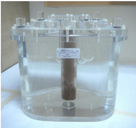
Figure 3. 6 Torso phantom with six hollow sphere inserts
