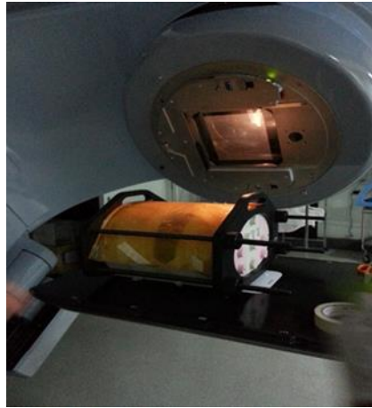
Figure 3.12 Dose measurement for tangential open beam plan in the CIRS thorax phantom
