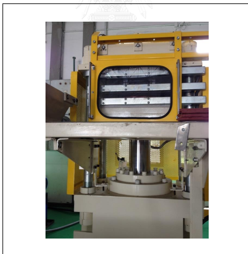
Figure 17: The electrically-heated hydraulic compression machine : PR2D-W500L500 PM (CHAREON TUT CO.,LTD)
