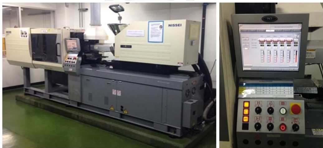
Figure 3.3 Injection molding for specimen preparation of ABS/UHMWPE blends
