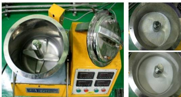
Figure 3.1 High speed mixer for mixing powder of ABS/UHMWPE blends
