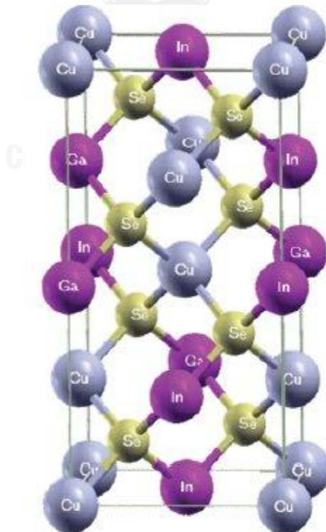
Figure 4 Crystal structure of chalcopyrite CIGS [19].
