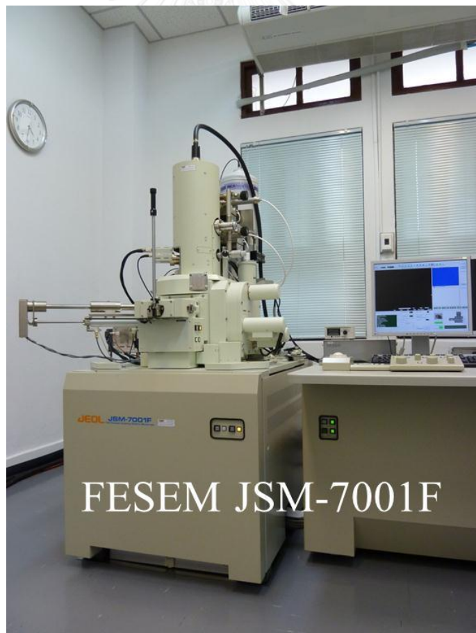
Figure 12 The image of JEOL JSM 7001 FESEM.
