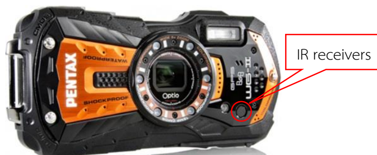
Figure C.9 Infrared (IR) receivers of Pentax Optio WG-2 digital camera
