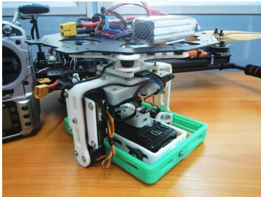
Figure 4.1 Developed 2-axis gimbal and data logger for Multicopter UAV (Drone)
