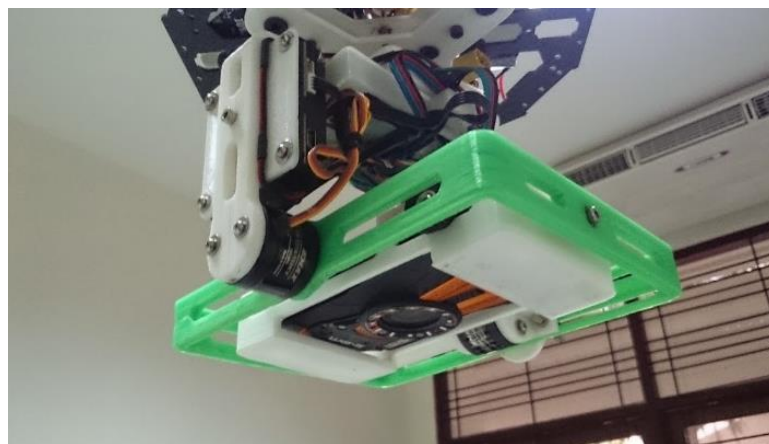
Figure E.5 The installation of a camera on gimbal frame
