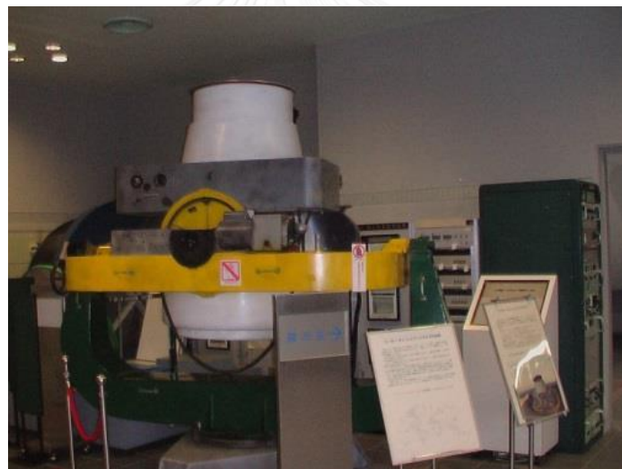
Figure 2.3 A Baker-Nunn satellite-tracking camera on an altitude-azimuth mount
