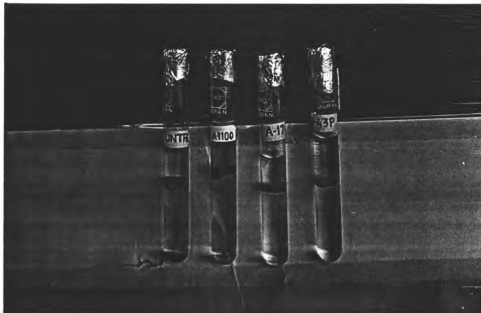
Figure 4.25 Existence of solvent extracted WF residue within the ethyl ether-water two layer system
