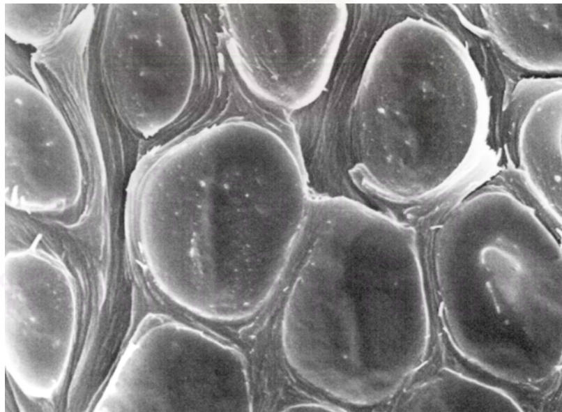
Figure 4.10 Scanning electron microscopy of transverse section of MAN-treated rubberwood cells (3,500X).
