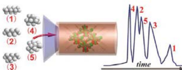
Figure 2.34 Schematic representation of the GC separation of alkanes with MOF-508; n -hexane (1); n -pentane (2); 2-methylpentane (3); 2-methylbutane (4); and 2,2-dimethylbutane (5). (88)
