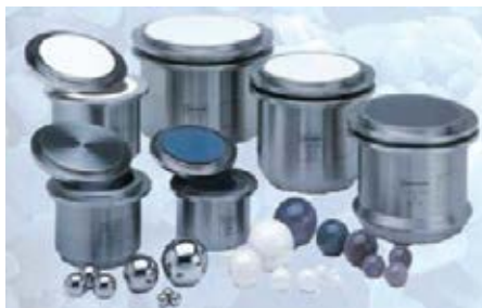
Figure 2.19 Ball mill: stainless steel vessel with a ball bearing. (12)
