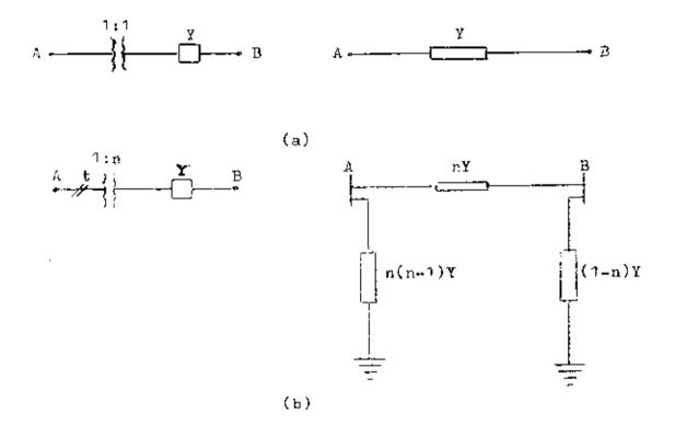
Fig. 2 Representation of a transformer
