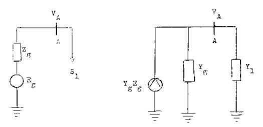
Fig. 1. Representations of a generator and of a load
