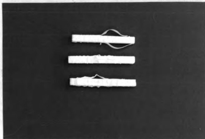
Figure 70. Peeling in TP bars coated with 100% MP.
