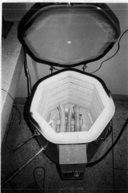
Figure 10. Electric furnace used for calcination.
