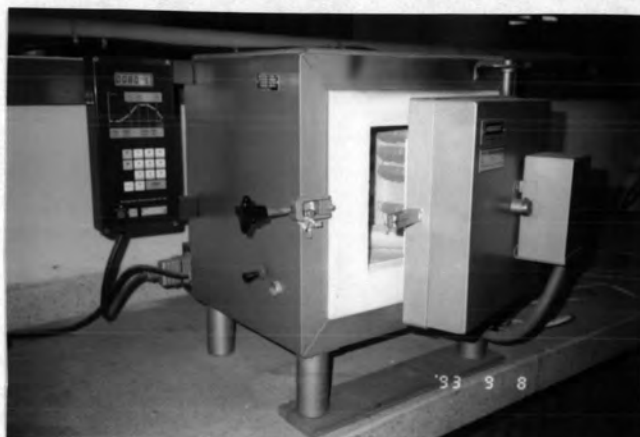
Figure 22. Electric furnace used for calcining compact bars.
