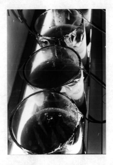
Figure 5 Cultivation of <u>Spirulina</u> in 15 l jar containing 10 l of medium. The aeration was provided by an air pump whereas illumination at 4,000 lux was provided by four white fluorescent lamps
