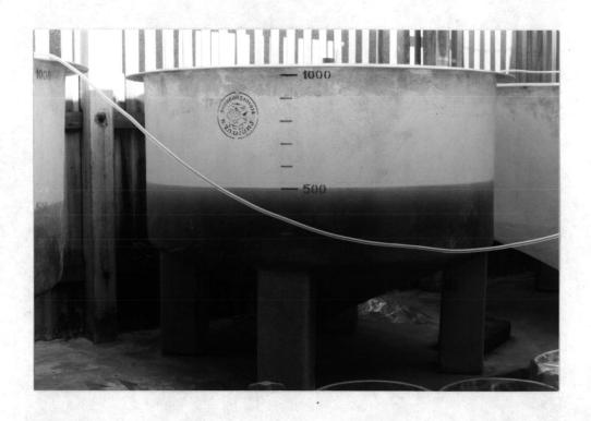
Figure 6 The outdoor cultivation of <u>Spirulina</u> on pilot scale with 500 l of medium
