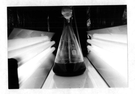
Figure 4 Cultivation of <u>Spirulina</u> in 4 1 flask containing 2 1 of medium. The aeration was provided by an air pump whereas illumination at 4,000 lux was provided by four white fluorescent lamps
