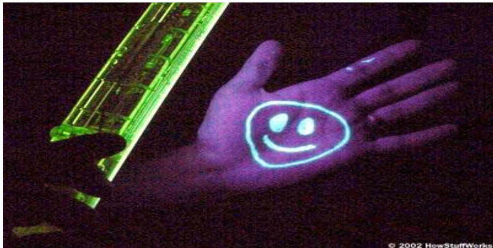
Picture 2.1: A picture of fluorescent tracer and black light
