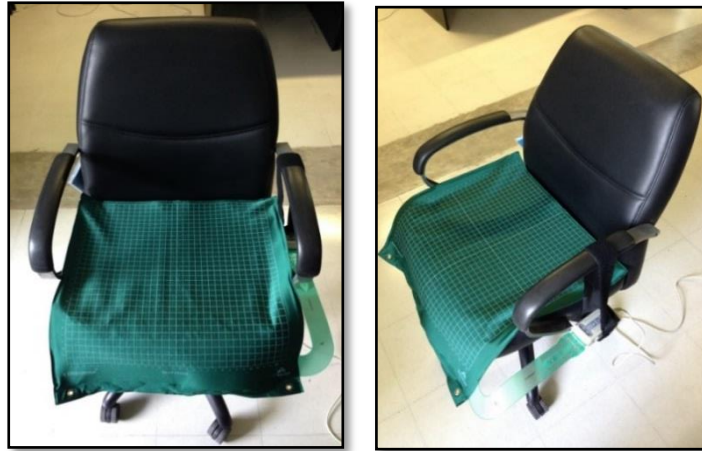
Figure 3.1 Seat pressure mat on the office chair
