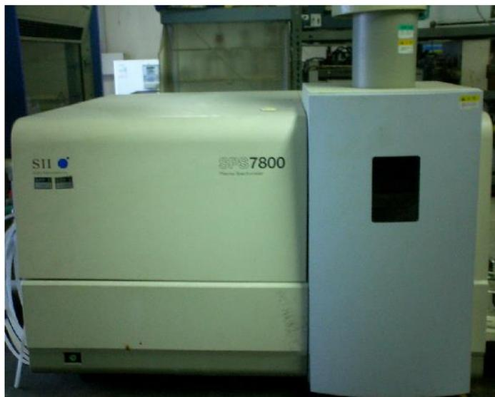
Figure A-3 Inductively Coupled Plasma-Atomic Emission Spectrometry (ICP-AES) (Seiko Instruments Inc., Ltd., SEIKO-SPS7800) at the Laboratory of Mineral Processing and Resources Recycling, Division of Sustainable Resources Engineering, Graduate School of Engineering, Hokkaido University, Japan
