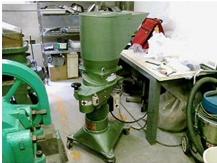
Figure 3. 8 Orient mill
