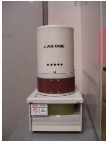
Figure 3. 4 ONE TPH-02 type low temperature grinding equipment
