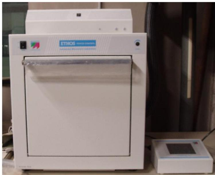
Figure 3. 5 Microwave digestion equipment (ETHOS PLUS)
