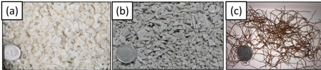
Figure 3. 9 Mixture of model samples; (a) ABS, (b) PVC, and (c) copper wires
