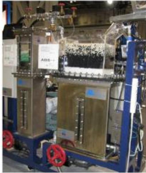
Figure 2. 13 Laboratory scale RETAC jig; batch (left) and continuous type (right)
