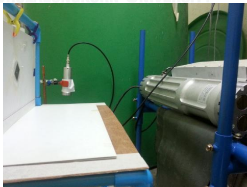
Figure 3.8 The experiment set up for the preliminary fast neutron radiography system with the use of lead sheet as the shielding material
