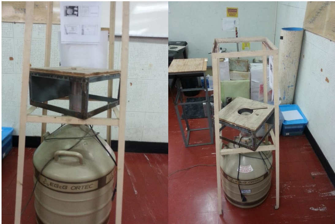
Figure 4-6 Mounting platform and support on top of LEPS-HPGe for heavy samples
