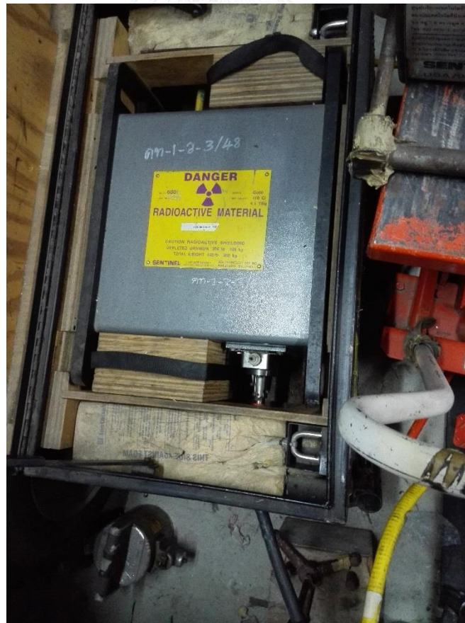
Figure 3-4 Cobalt-60 radiography projector (Sentinel 680B) at NDT Division of the Nuclear Technology Service Center of Thailand Institute of Nuclear Technology
