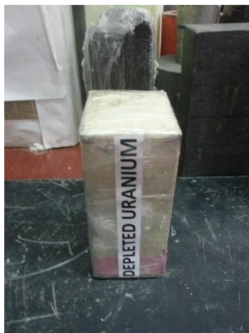
Figure 3-2 Depleted Uranium block
