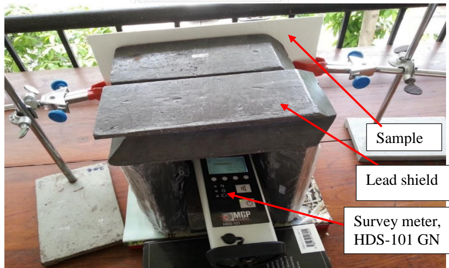
Figure 3. 10: The in situ measurement using the survey meter of the HDS-101 GN
