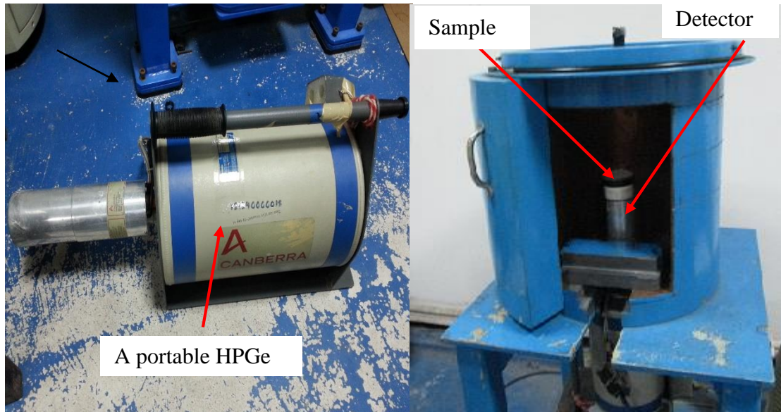
Figure 3. 3: Lead shield to lower gamma background level
