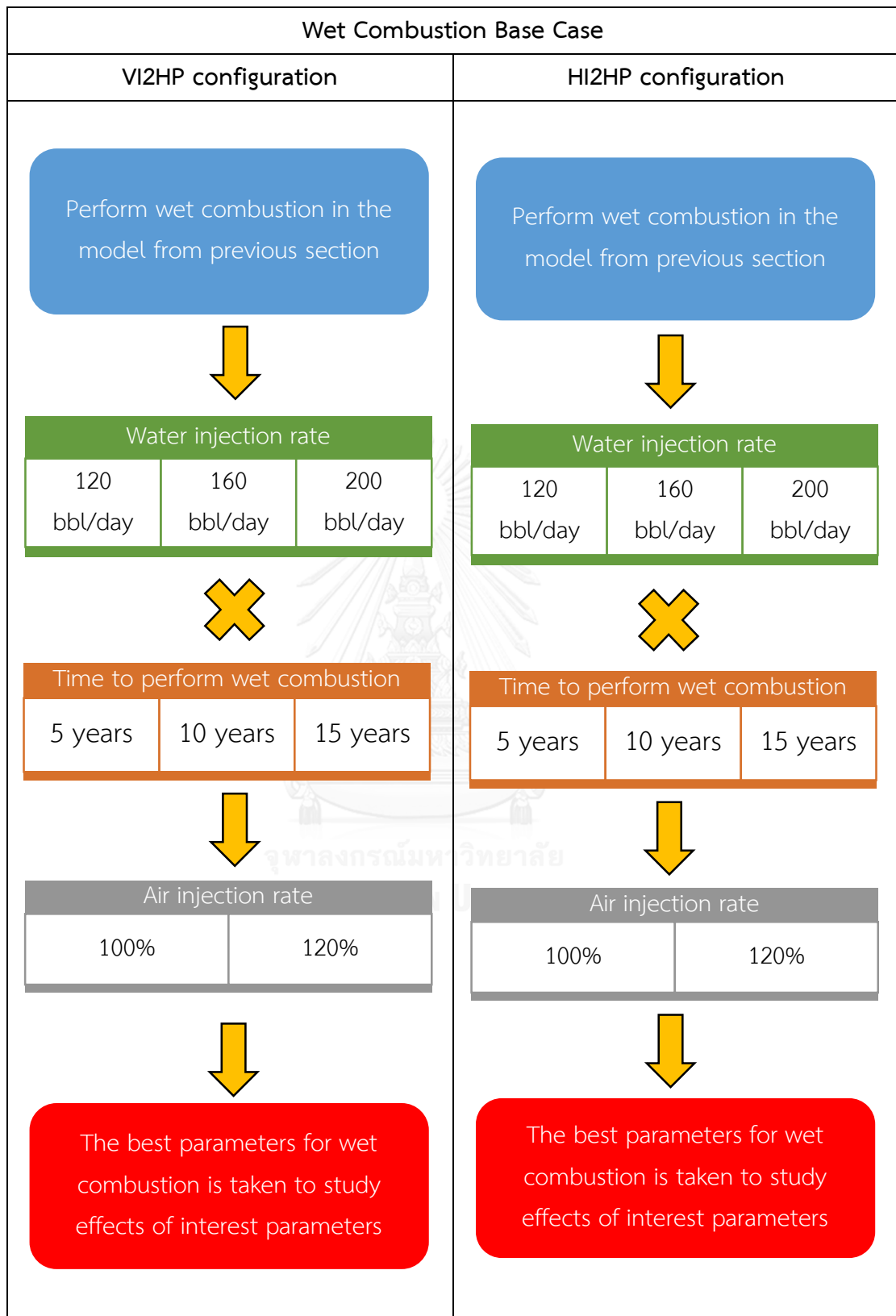
Figure 4.15 Flow chart of methodology for identification of wet combustion base case model
