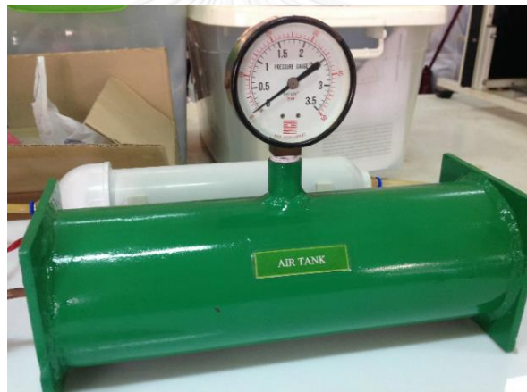
Figure 3.6 The pressure gauge
