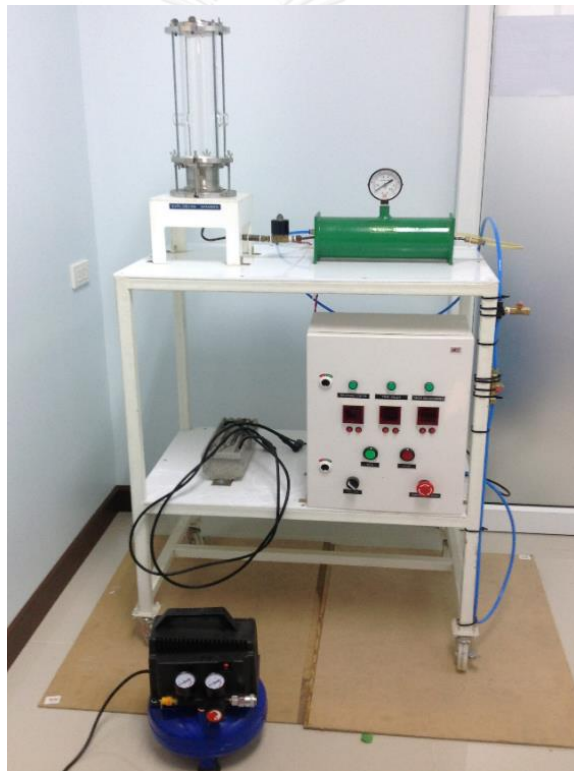
Figure 3.4 The compressed air and pipes of compressed air section.
