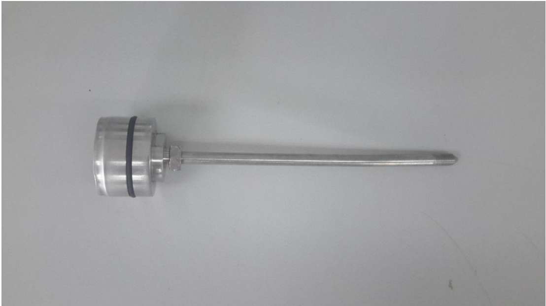
Figure 4.13 Fixed length outlet tube at the outlet of core holder
