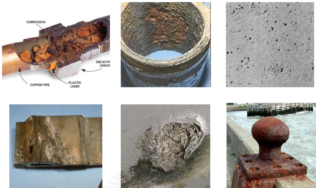
Figure 2.14 Types of corrosion: (a) Galvanic corrosion, (b) Concentration cell corrosion, (c) Pitting, (d) Stress corrosion cracking, (e) Intergranular corrosion and (f) Uniform corrosion attacks [24]
