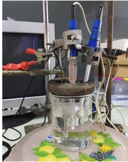
Figure 3.5 The electrochemical Tafel slope analysis apparatus
