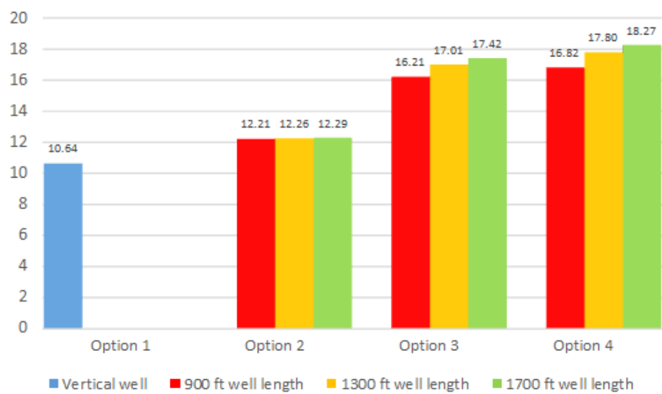
Figure 5.6 Recovery factor for different well types for well arrangement option 1 when dumping water from a strong aquifer
