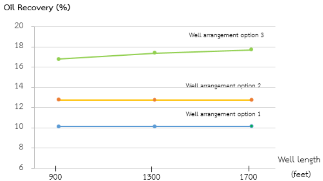
Figure 5.18 Oil recovery factor for different horizontal well length for vertical producer and horizontal dumper for intermediate aquifer (10 PV)
