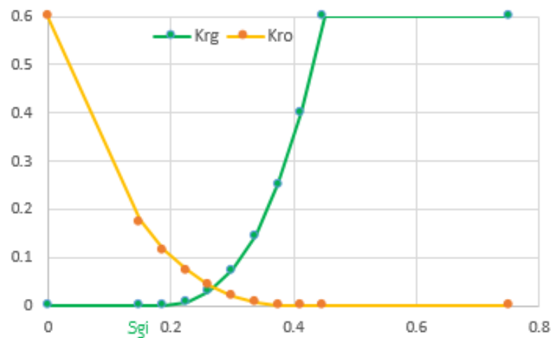
Figure 4. 5 Gas-oil relative permeability curves
