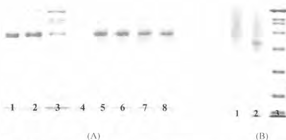
Figure 3.5 SDS-PAGE of (A) Lanes 1 and 2: unprocessed BSA, Lane 3: molecular weight standards, broad range (Bio-Rad Laboratories, Hercules CA, USA), Lane 4: sample buffer, Lanes 5 and 6: BSA recovered from 10% w/w BSA-loaded LCS microparticles, prepared at a spray rate of 3 ml/min and the inlet air temperature of 120 °C and 100 °C, respectively, Lanes 7 and 8: BSA recovered from 5% w/w BSA-loaded LCS microparticles, prepared at a spray rate of 3 ml/min and the inlet air temperature of 120 °C and 100 °C, respectively, and (B) Lane 1: blank chitosan microparticles, Lane 2: BSA recovered from 1% w/w BSA-loaded LCS microparticles, prepared at the spray rate of 3 ml/min and the inlet air temperature of 120 °C, and Lane 3: molecular weight standards, broad range
