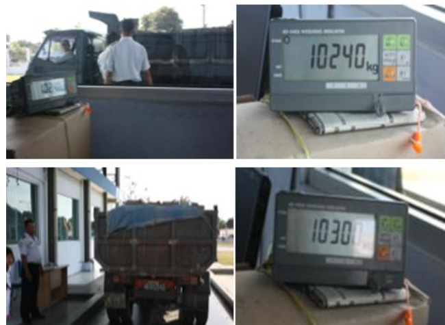
Figure 6.8 Measurements of Weight at the Weighbridge
