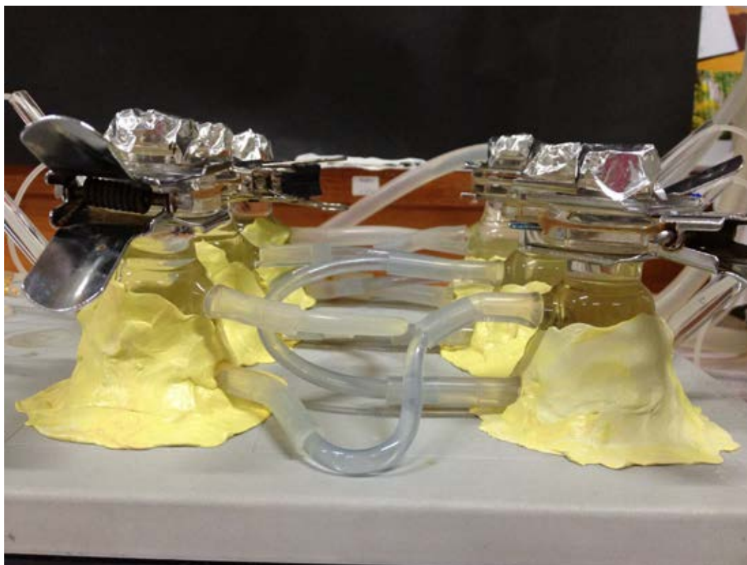
Figure 3D The excised pig ear skin was placed between the donor and the receptor compartment of Franz diffusion cell.
