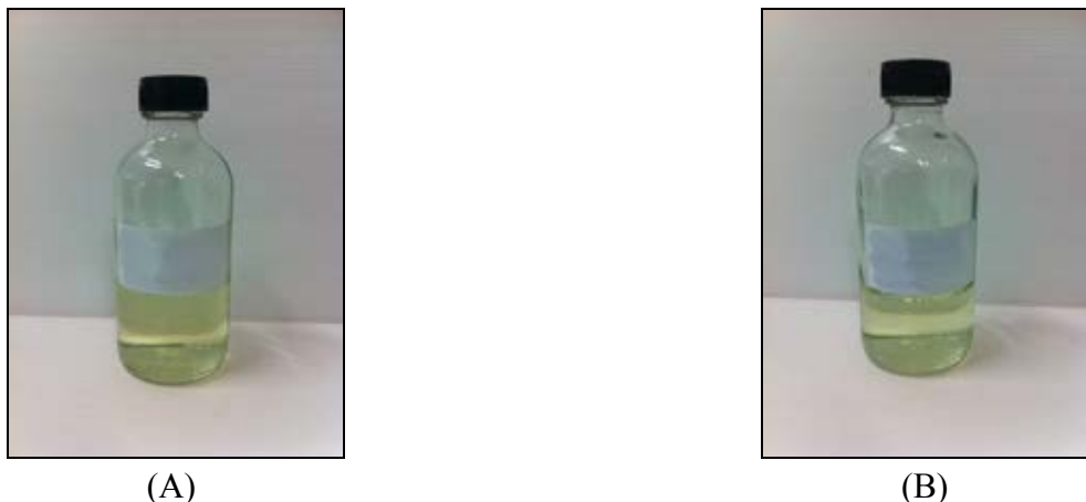
Figure 4-19 GS HCl formulation prepared with DG and sodium metabisulfite tartrate buffer pH 3 under light (A) in the dark (B) after 7 days of storage
