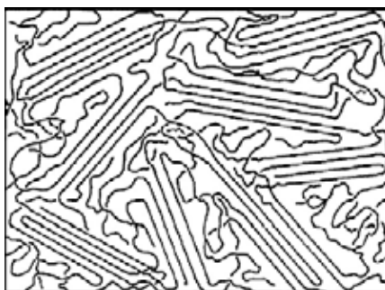
Figure 2.12 Crystalline (ordered)-amorphous (disorder) or heterogeneous structure of Polyaniline [7]
