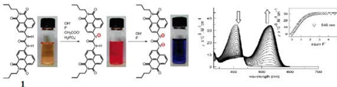
Figure 1.4 The changes in color (Left) and the changes in the absorption spectra (Right) of 1 upon addition of fluoride in DMSO [9].
