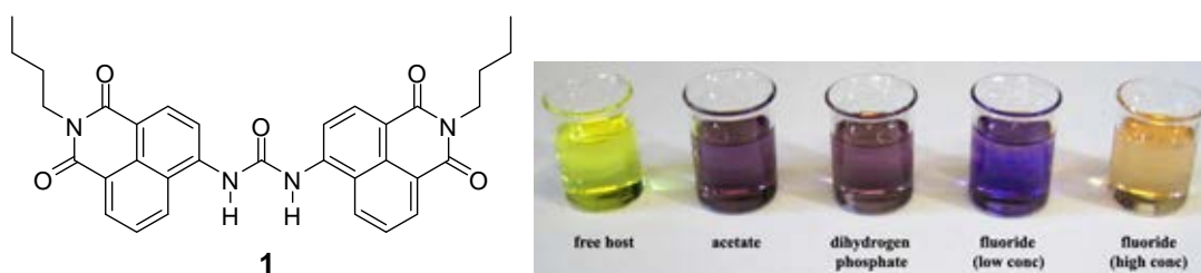
Figure 1.3 Compound 1 and the change in color of 1 in DMSO upon addition of various anions [10].
