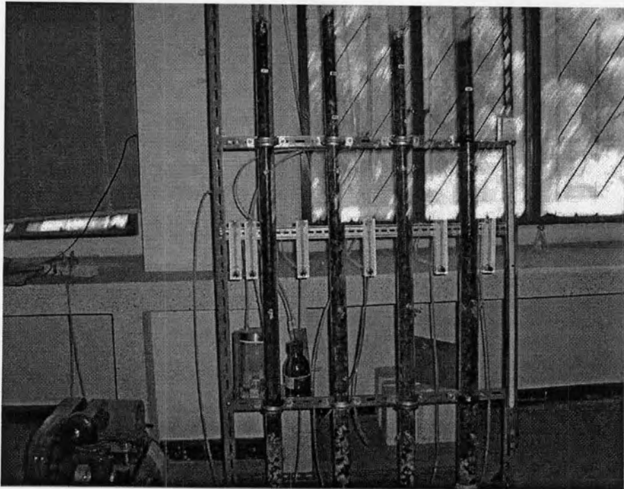
Figure B-11 Four Column of Biofilters
