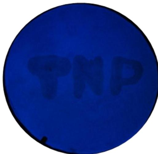
**Figure 3.15** Glc-DHP 1 fluorescent paper sensor for TNP visual detection by handwriting on the paper using TNP solution (40  $\mu\text{M}$ ) as ink. The digital image was taken under a UV lamp (365-nm irradiation).
