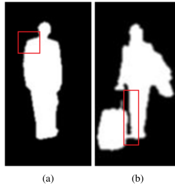
Figure 3.15: (a) Failure of detecting shoulder and (b) leg as carried objects due to its steady signal in time-series graph.
