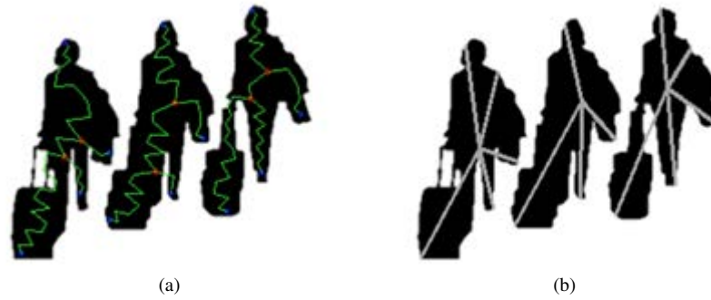
Figure 3.13: (a) Limb points of triangle-based skeleton vary in a wide range from each frame while (b) limb points of star skeleton are more stable
