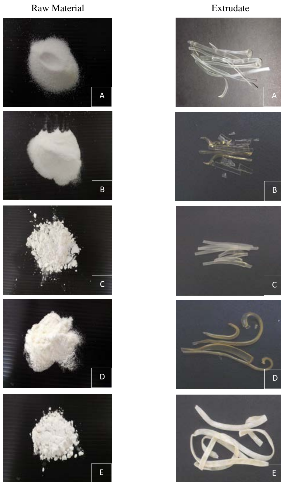
Figure 4-14 Raw materials and extrudates of 50:50 drug/polymer from hot-melt extrusion; A) Soluplus ® ; B) Kollidon ® VA-64; C) Eudragit ® EPO; D) Kollidon ® K-30; E) HPC
