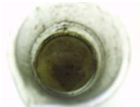
Figure 9.3 (a) liquid product sample from the supercritical water reforming of glycerol with 10 wt.% \text{Co}/\gamma\text{-Al}_2\text{O}_3 catalyst at 748 K (b) solid products after filtration
