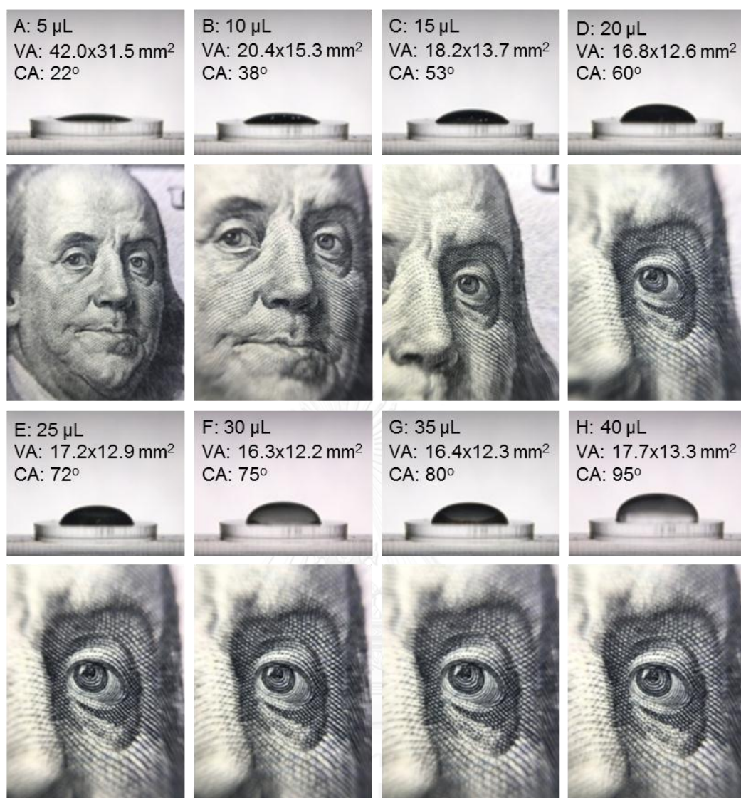
Figure 4.6 Microscopic images of the Benjamin Franklin's eyes on the front side of a new USD100 banknote were taken by an iPhone 6s Plus coupled with the 6-mm ePDMS plano-convex lens of various focal lengths fabricated by dispensing (A) 5 \mu\text{L} , (B) 10 \mu\text{L} , (C) 15 \mu\text{L} , (D) 20 \mu\text{L} , (E) 25 \mu\text{L} , (F) 30 \mu\text{L} , (G) 35 \mu\text{L} , and (H) 40 \mu\text{L} IPDMS. The viewing area (VA, 4:3 format) and contact angle (CA) were indicated in the images.
