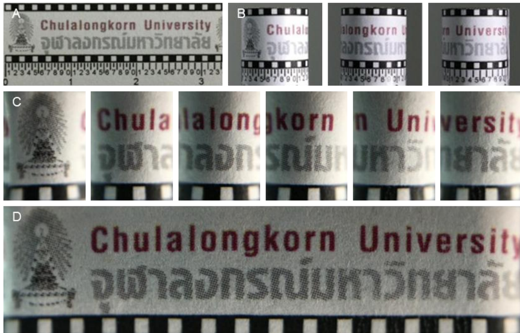
Figure 4.15 Photographic images of a printed-paper strip as it: (A) was laid on a flat surface and (B) was wrapped around a 10 mm cylinder. (C) Microscopic images of the curved paper strip and (D) the corresponding panorama microscopic image of the curved paper strip taken by an iPhone 6s Plus coupled with a 3-mm lens (see Figure 4.14).
