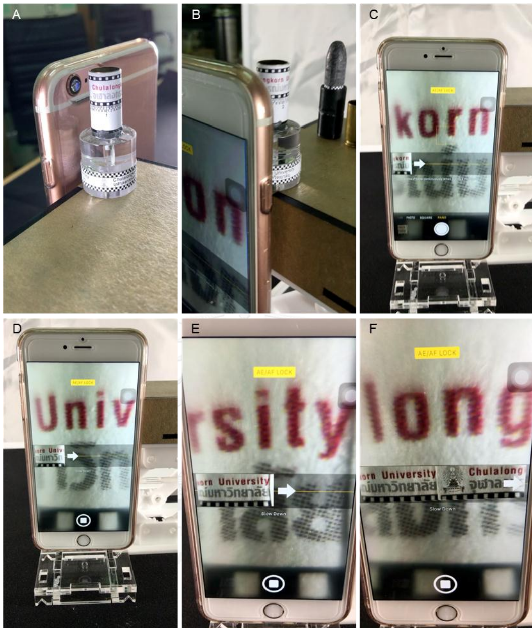
Figure 4.14 A series of still images show an experiment setup and panorama microscope imaging using a smartphone microscope equipped with a 5-mm ePDMS plano-convex lens and homemade rotating device. The device was rotated at 3 rpm while smartphone microscope taking panorama image of the 3.3 mm x 1.4 mm paper strip wrapped around a 10 mm cylinder. The panorama app stitched the images on-the-fly.
