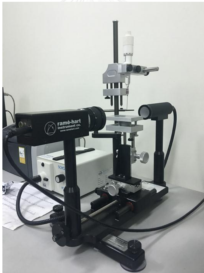
Figure 3.3 Photographic image of the contact angle measurement.
