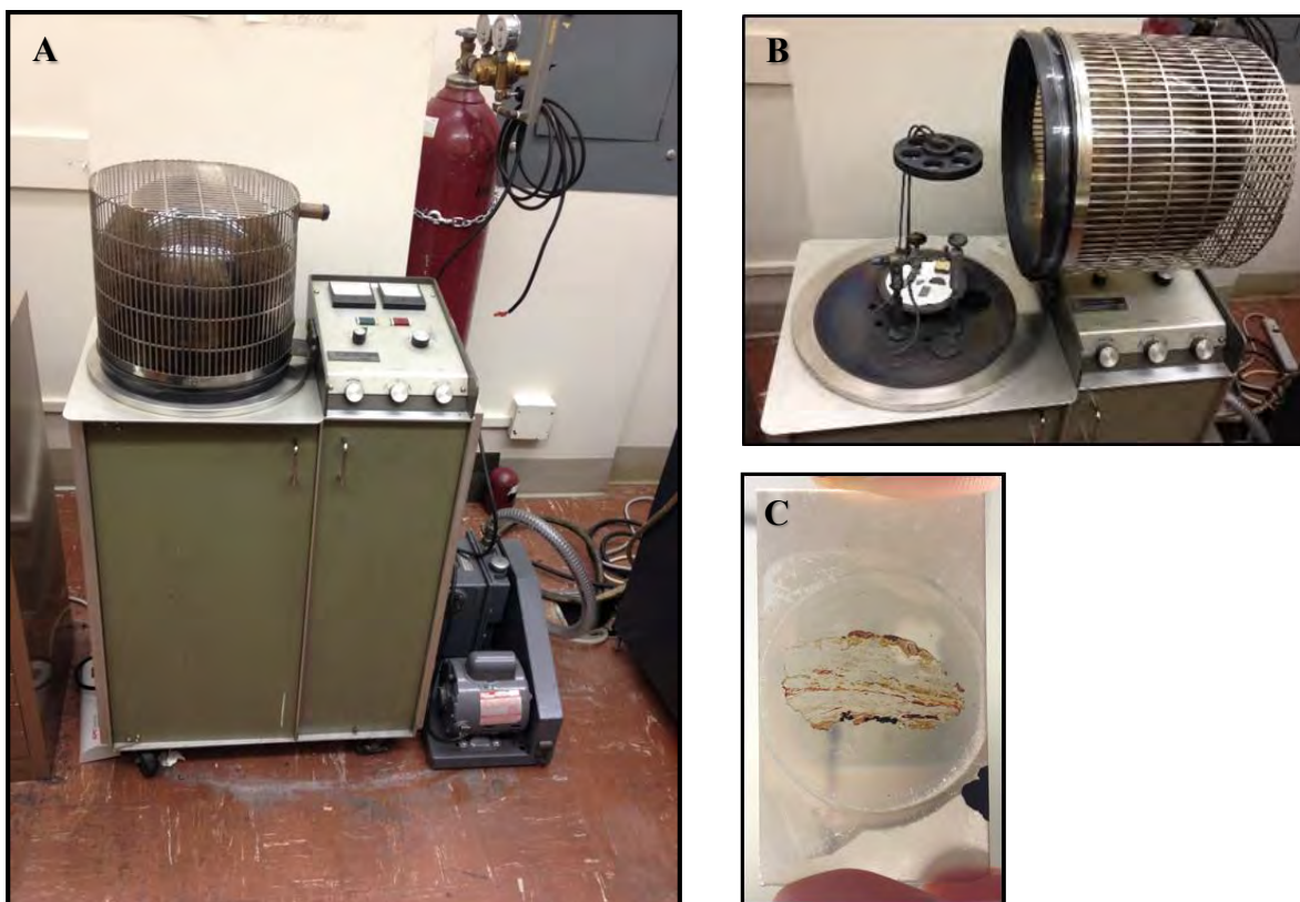
Figure 2.6 Carbon coating equipment (A) Carbon coating equipment, (B) The inside of Carbon coating equipment and (C) Polished thin section, coated with carbon
