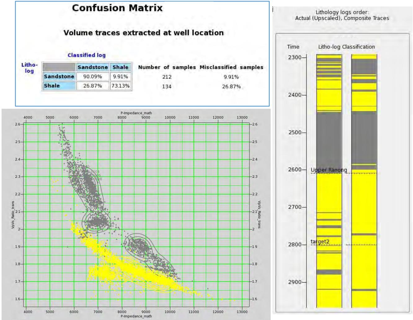
Figure 3.18 The probability density function distribution of sandstone and shale.
