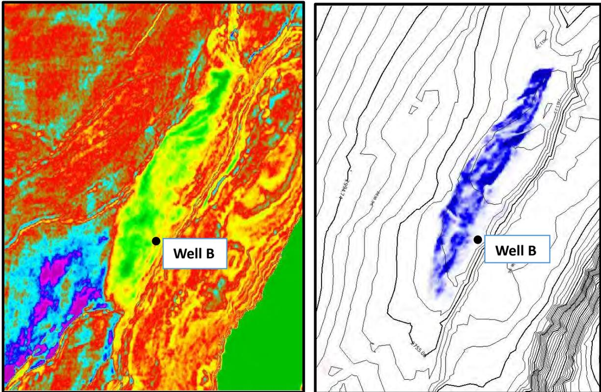
Figure 4.4 The comparison between acoustic impedance map and AVO attribute map which close up to well B gas reservoir showing acoustic impedance map is more adjacent to fault plane.
