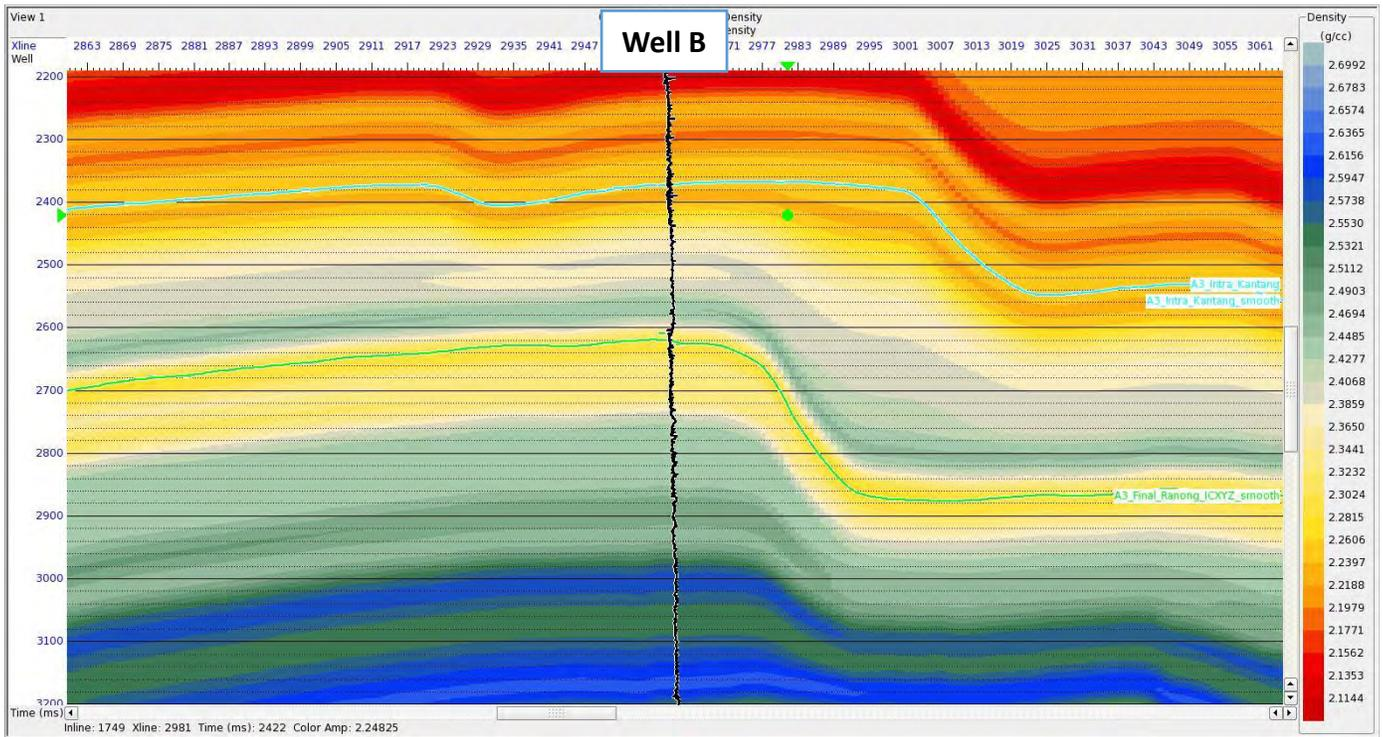
Figure 3.14 The inline section of low frequency density model.
