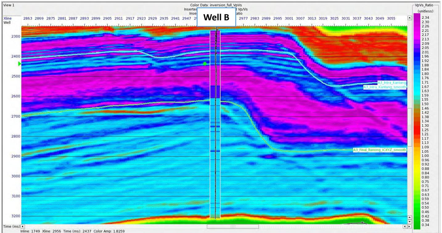
Figure 3.17 The inline section of inverted Vp Vs ratio.
