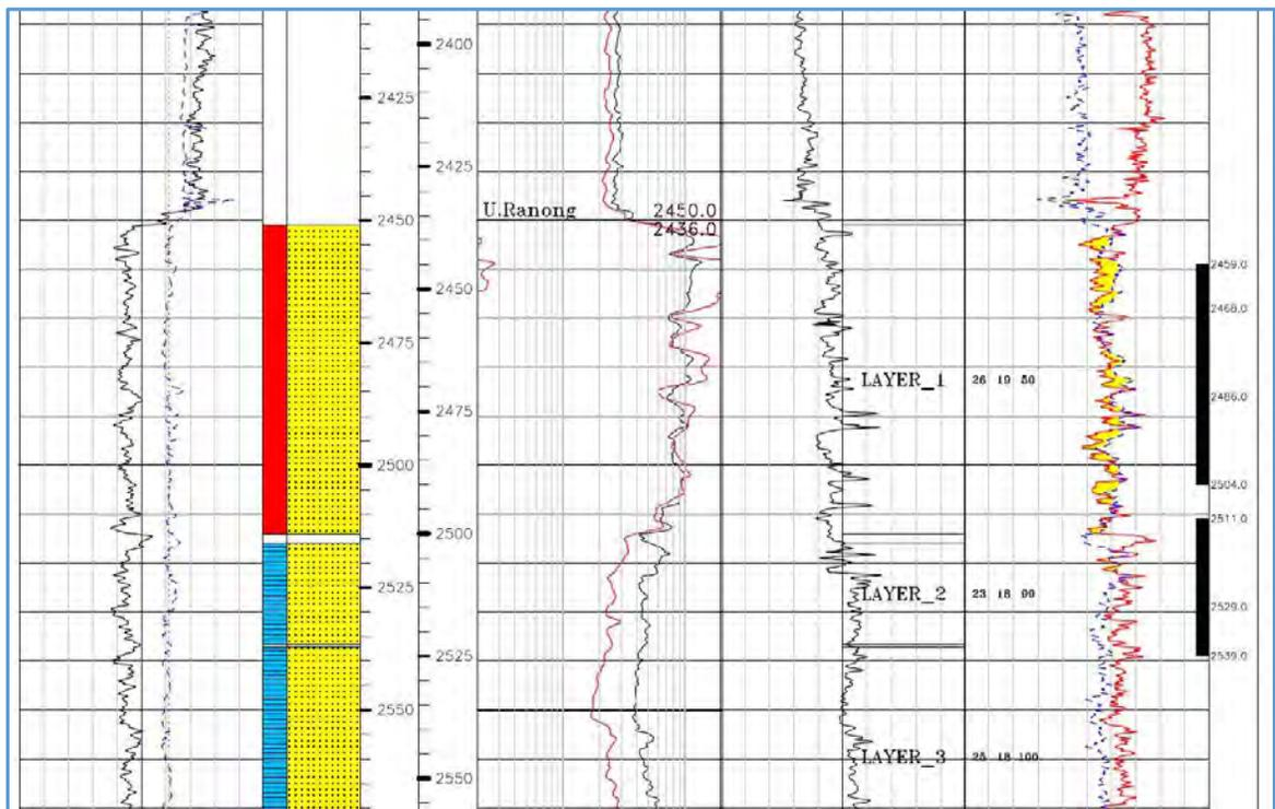
Figure 1.3 The depth location of gas reservoir in well B
