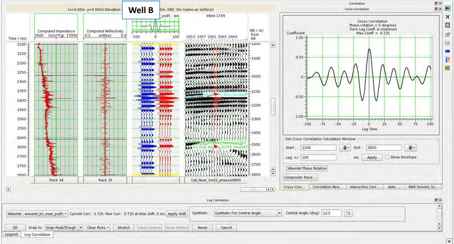
Figure 3.8 Log correlation window of seismic near angle stack.
