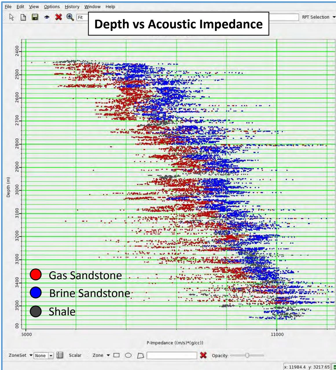
Figure 3.3 Cross-plot showing depth trend of acoustic impedance.
