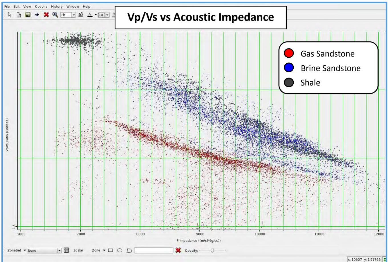
Figure 3.5 Cross-plot showing Vp Vs ratio against acoustic impedance.
