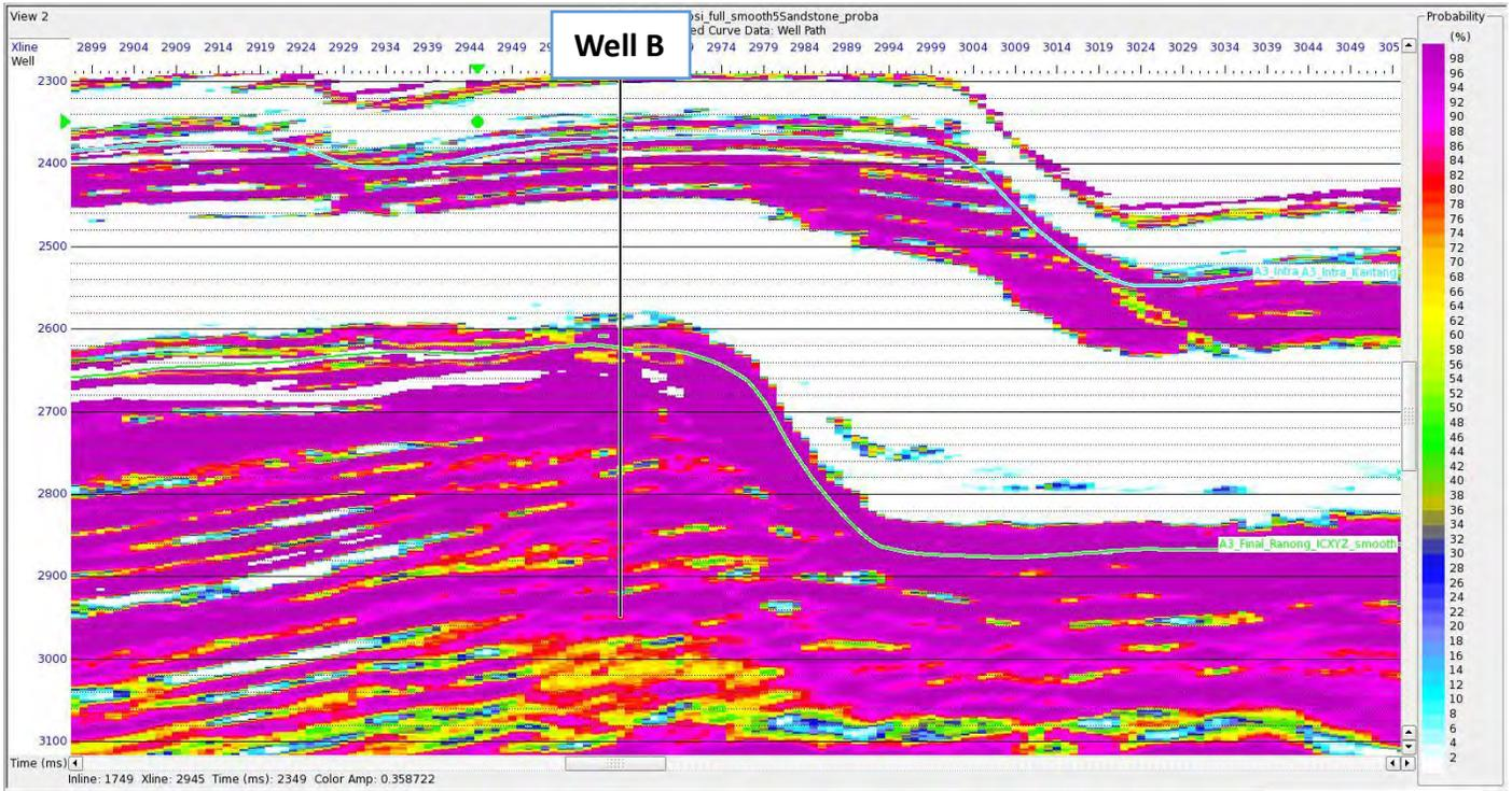
Figure 3.20 The inline section of probability of sandstone volume.
