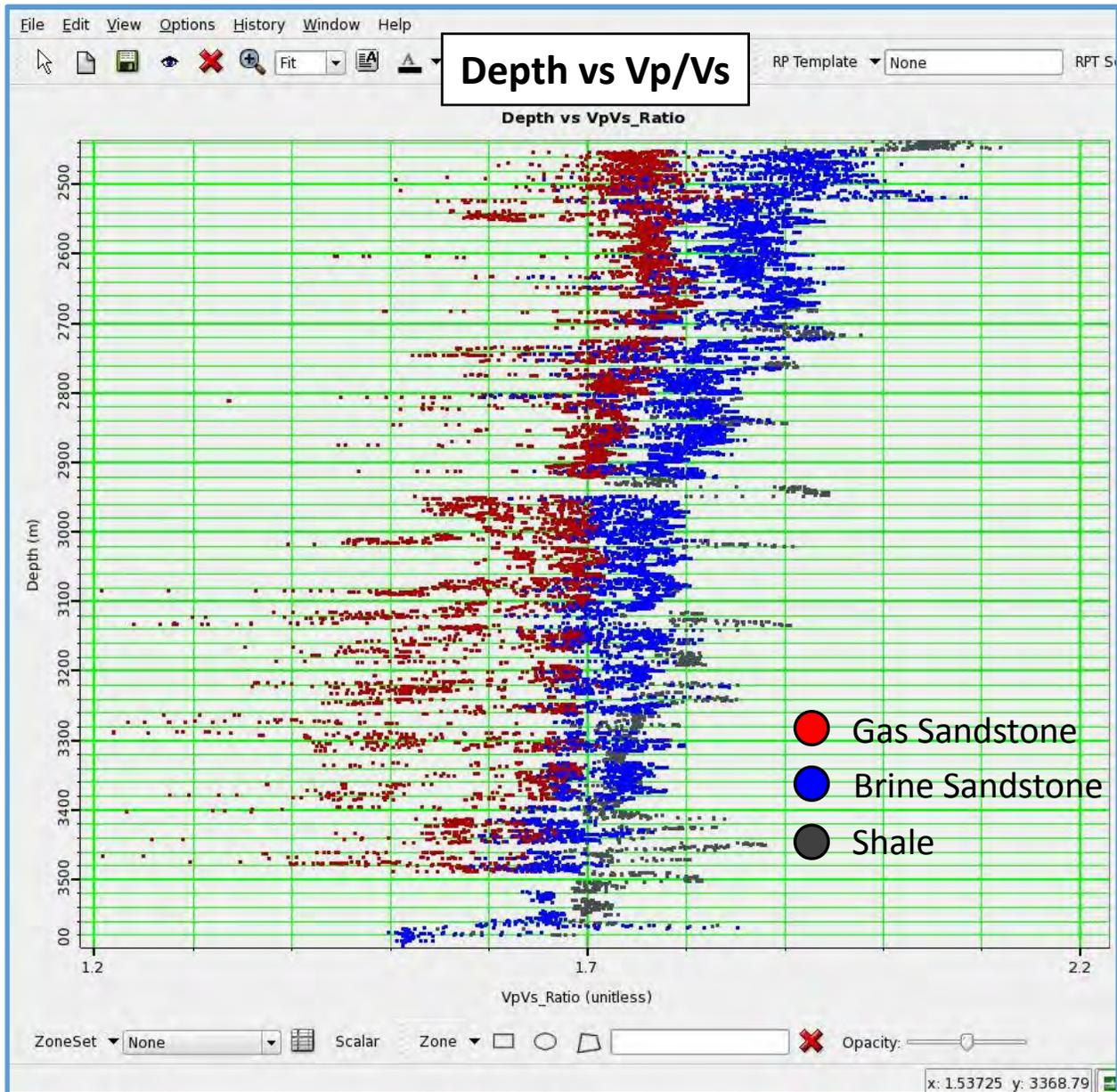
Figure 3.4 Cross-plot showing depth trend of Vp Vs ratio.
