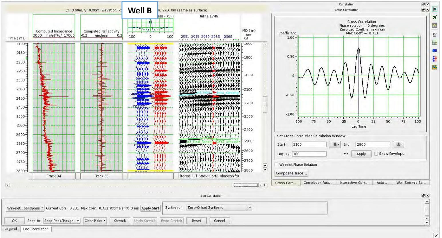
Figure 3.7 Log correlation window of seismic full offset stack.
