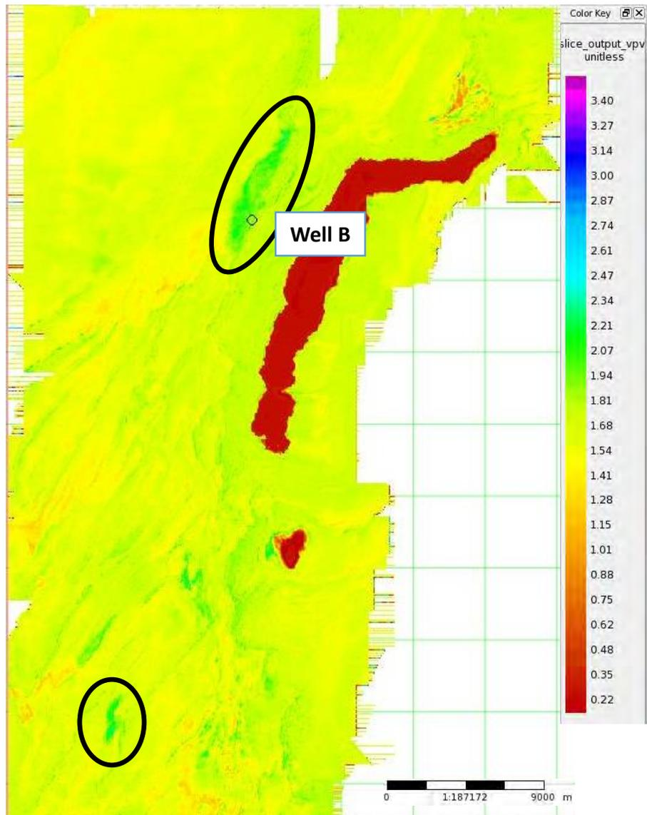
Figure 4.2 Vp Vs ratio slice map along horizon showing 2 anomaly zones that might quantitatively be gas reservoirs.
