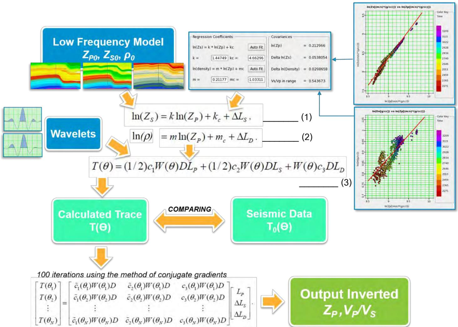
Figure 2.2 The process of simultaneous inversion.
