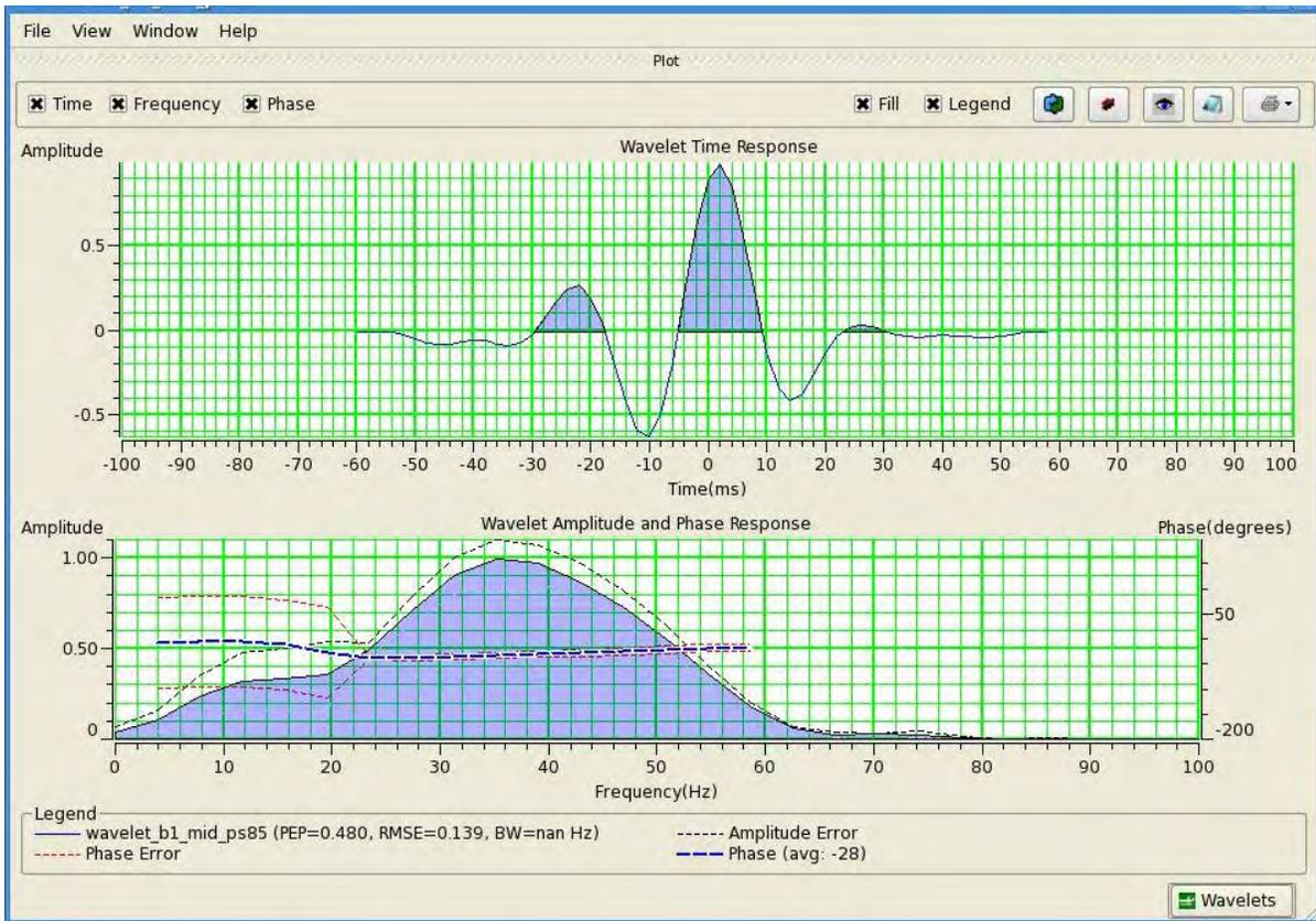
Figure 3.11 The wavelet estimation of seismic mid angle stack.
