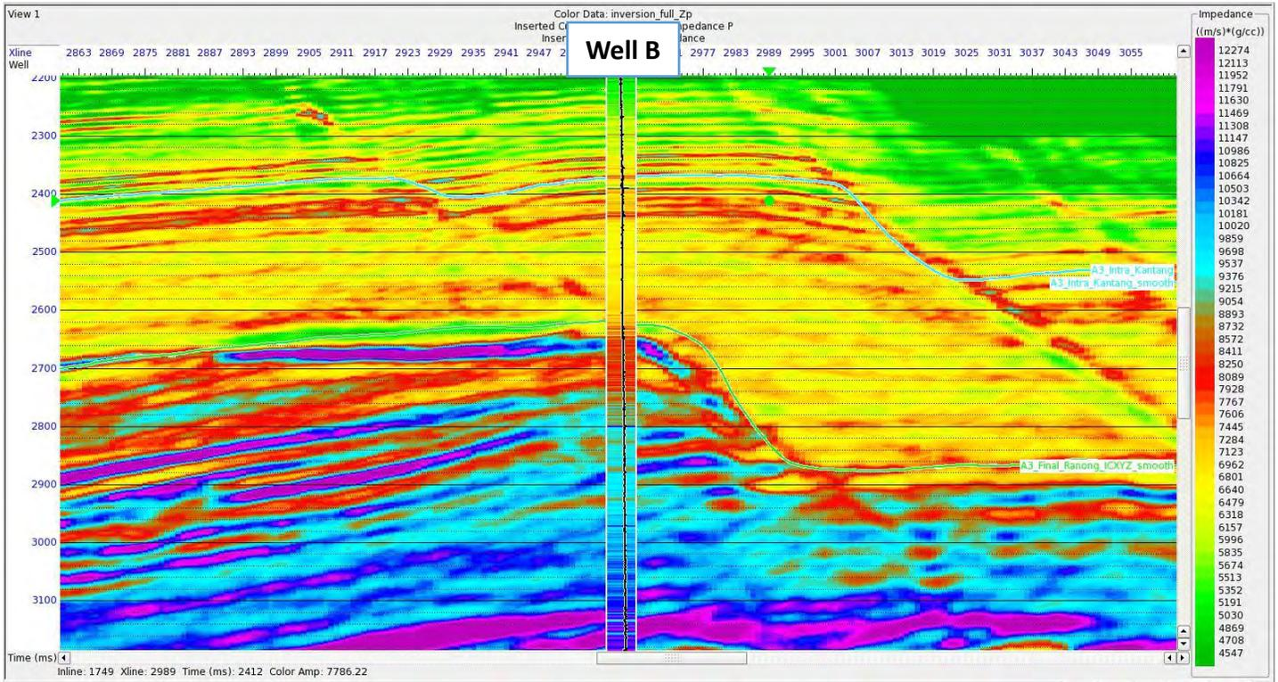
Figure 3.16 The inline section of inverted acoustic impedance.
