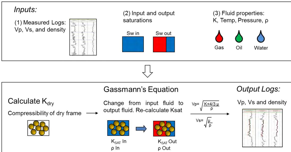
Figure 2.1 The concept of fluid replacement model.
