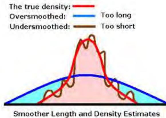
Figure 2.4 The schematic of smoother process.
