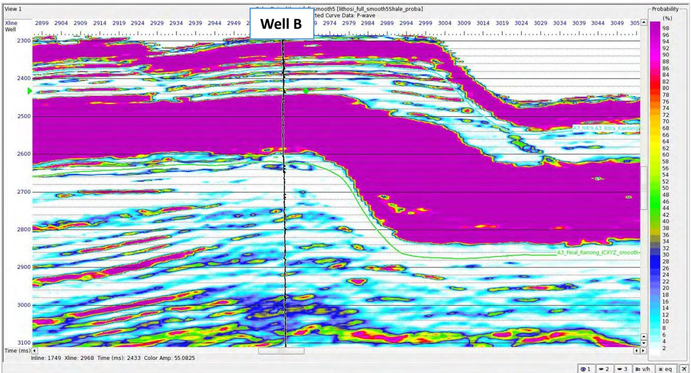
Figure 3.21 The inline section of probability of shale volume.
