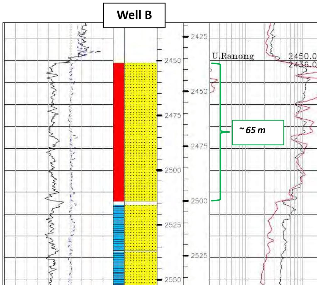
Figure 3.6 The thickness of gas sandstone at well B.
