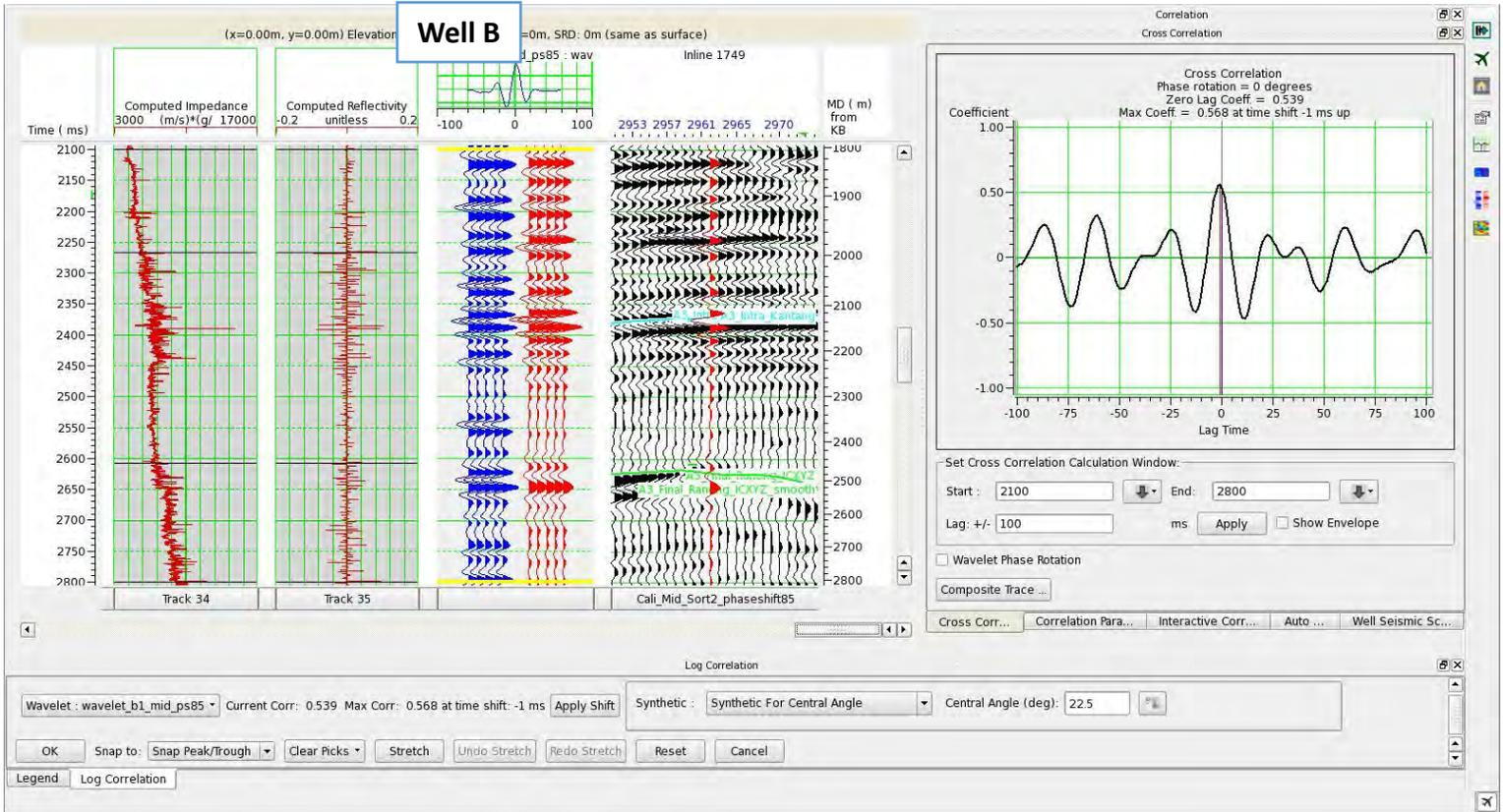
Figure 3.9 Log correlation window of seismic near angle stack.
