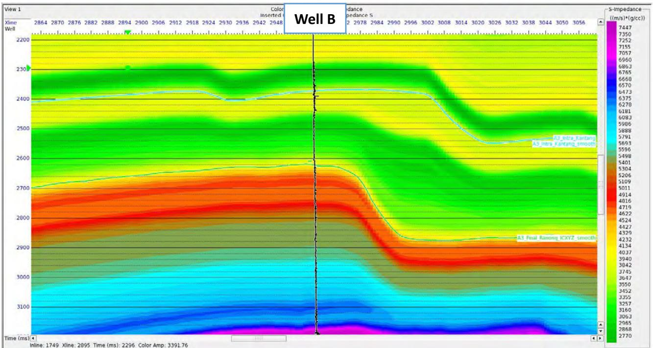
Figure 3.13 The inline section of low frequency shear impedance model.
