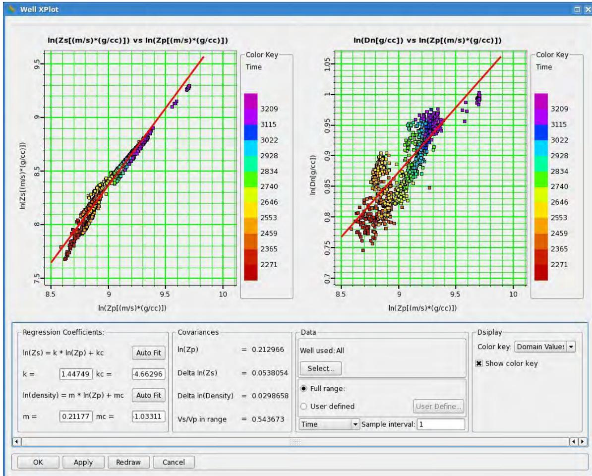
Figure 3.15 The parameter using in simultaneous inversion.
