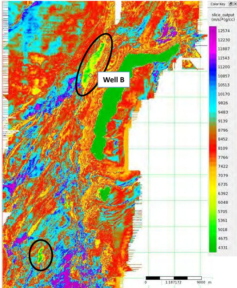
Figure 4.1 Acoustic impedance slice map along horizon showing 2 anomaly zones that might quantitatively be gas reservoirs.
