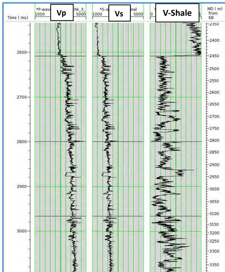
Figure 3.1 The predicted shear wave velocity log.
