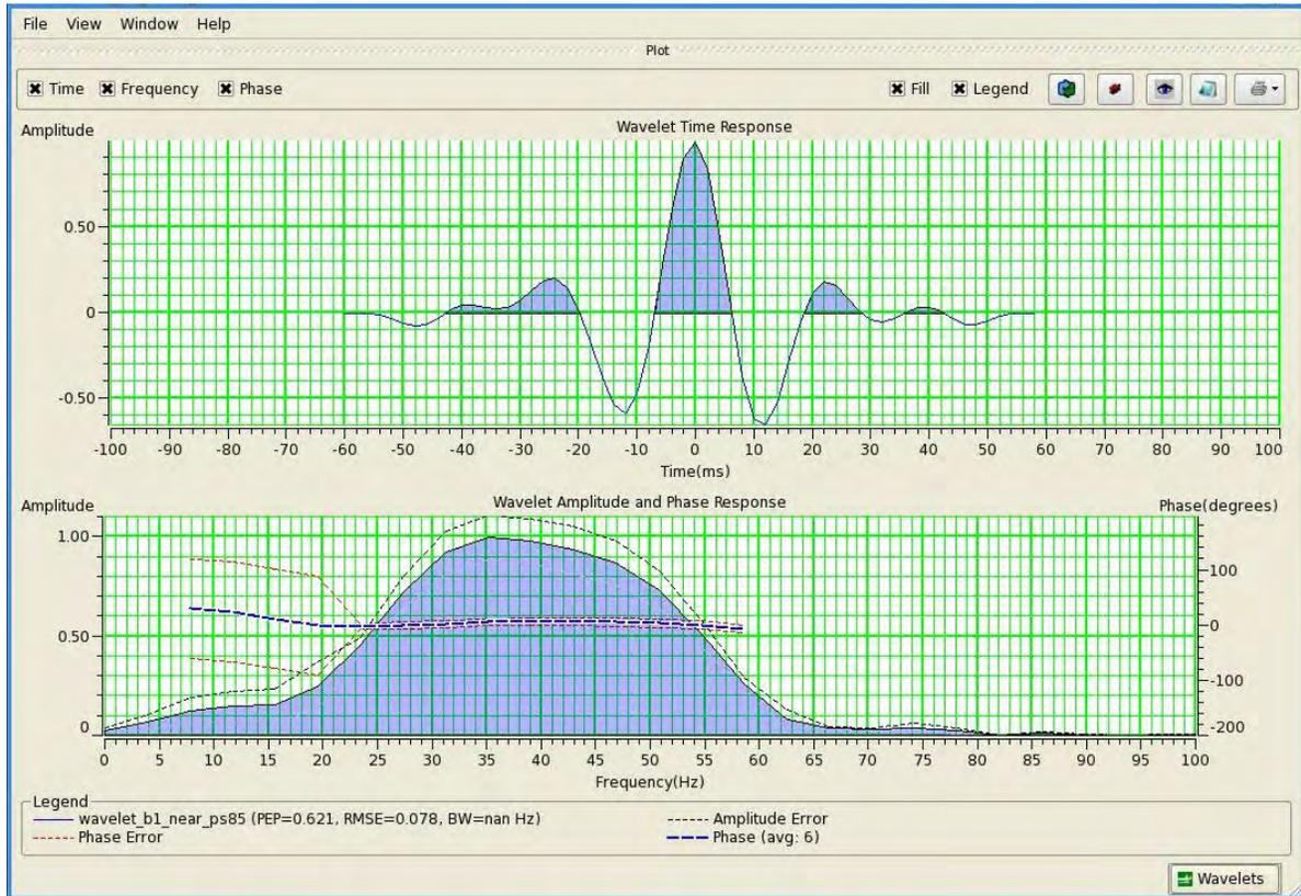
Figure 3.10 The wavelet estimation of seismic near angle stack.
