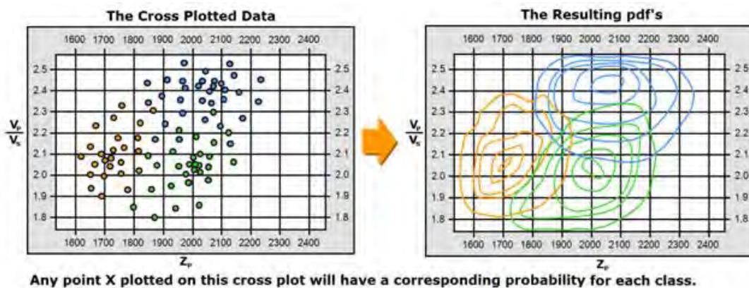
Figure 2.3 The concept of probability density function (pdf).
