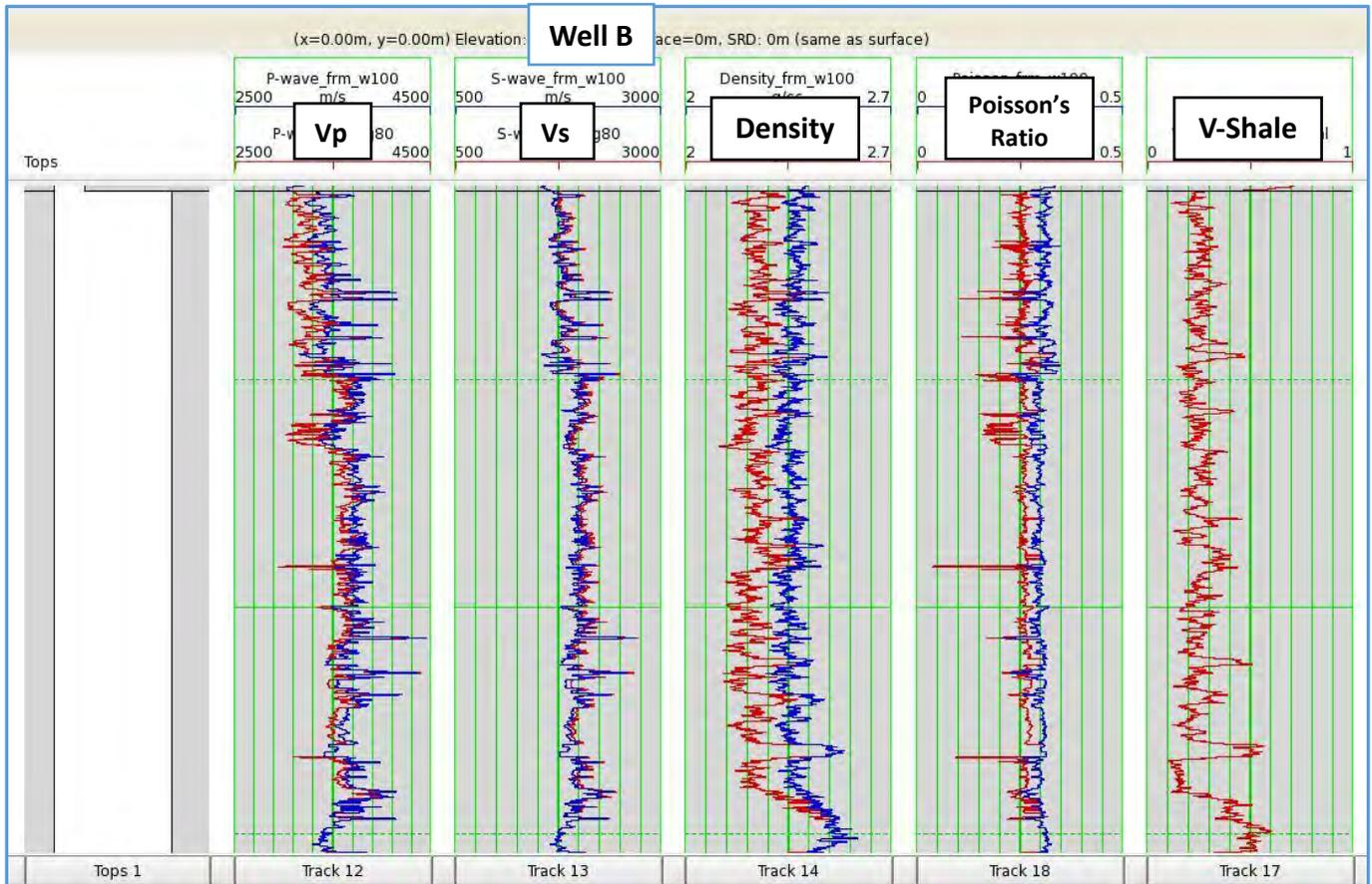
Figure 3.2 The log data of fluid replacement model in case of 80% gas sandstone and 100% brine sandstone.
