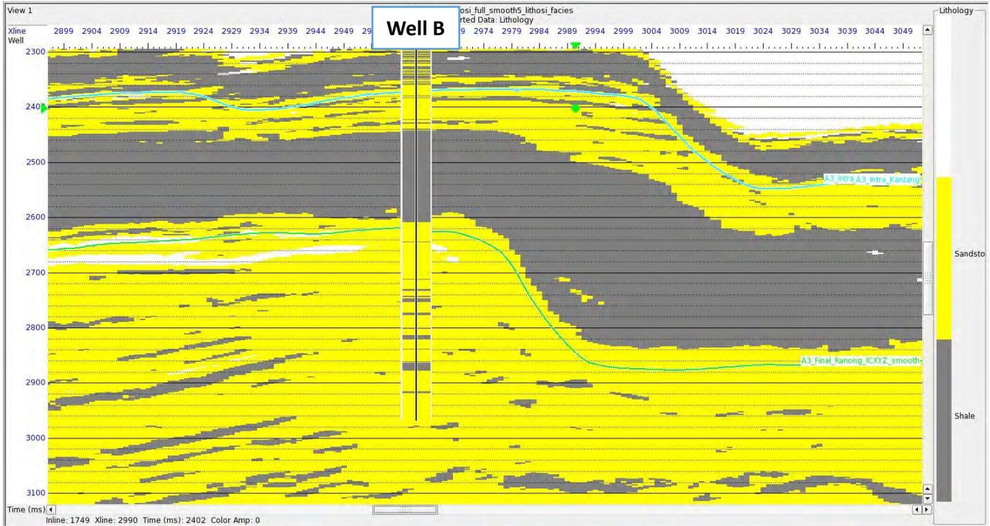
Figure 3.19 The inline section of lithology volume of sandstone and shale.
