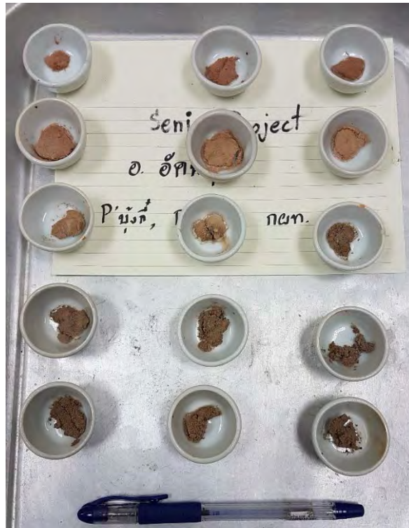
Figure 2.2 Samples in crucibles (the furnace can hold up to 15 samples at a time)
