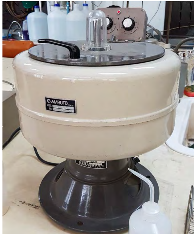
Figure 2.6 A centrifuge machine. It can hold up to 4 tube at a time.
