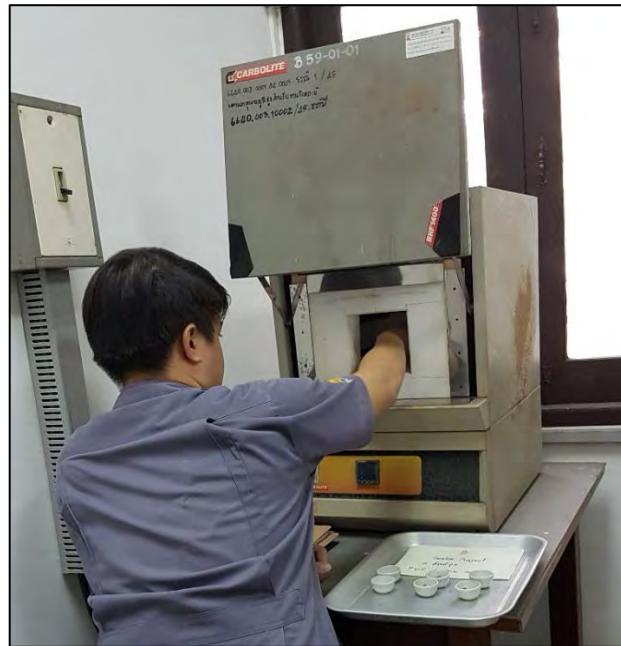
Figure 2.4 15 Samples being place in a furnace
