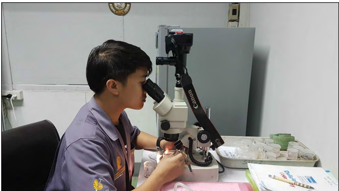
Figure 2.9 Macrofossils are being picked using a stereo microscope and forceps.
