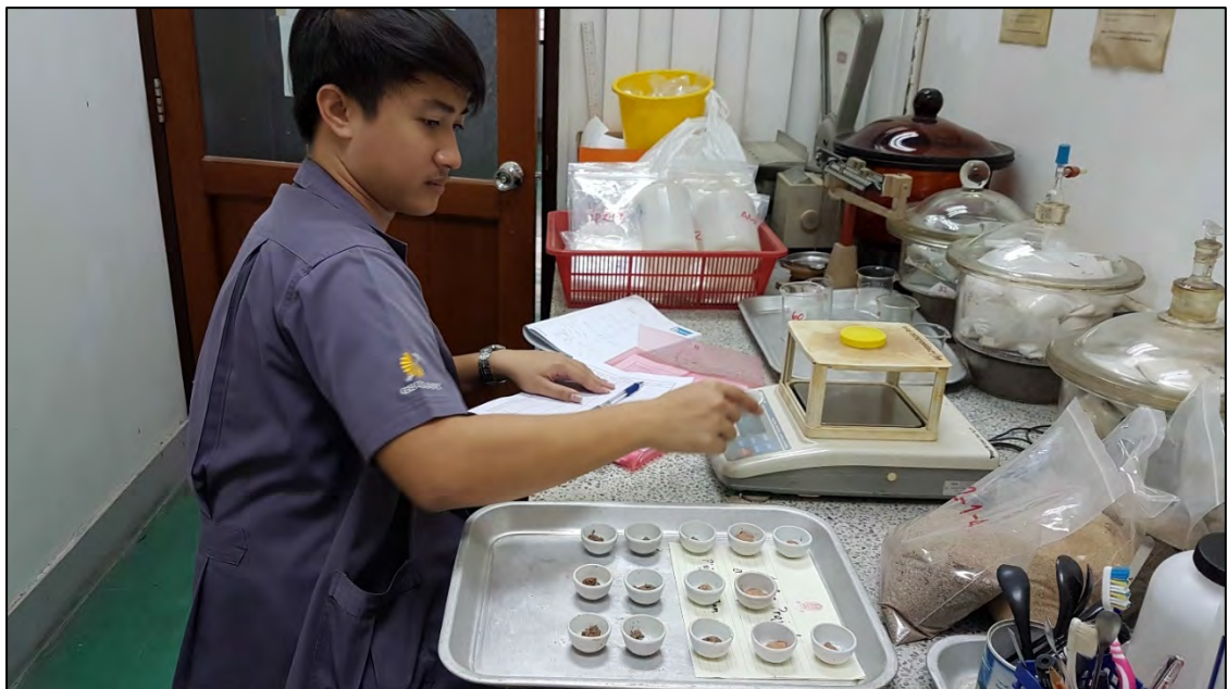
Figure 2.3 Samples must be weighed after drying and heating up to 550 °C and 950 °C.
