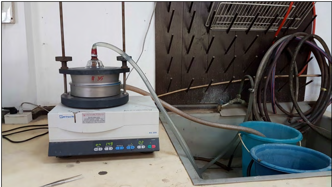
Figure 2.8 A samples being wet-sieved with a 500 µm mesh to separate macrofossils.
