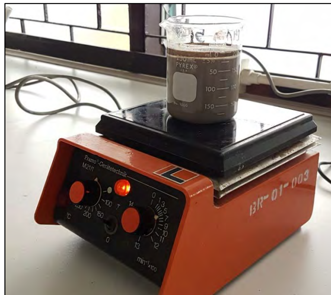
Figure 2.7 A sample are being stirred with magnetic stirrer in 5% Calgon to disperse the sediment particle.
