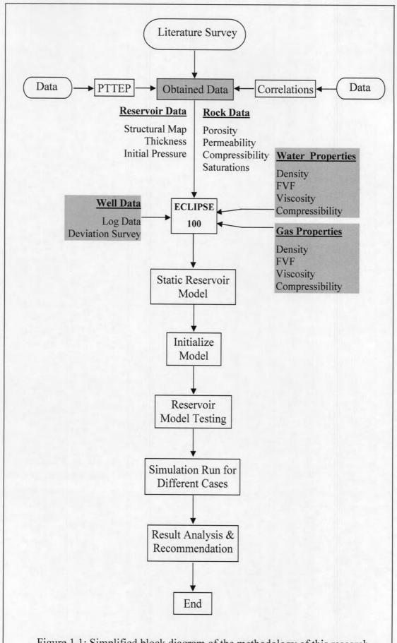
Figure 1.1: Simplified block diagram of the methodology of this research.
