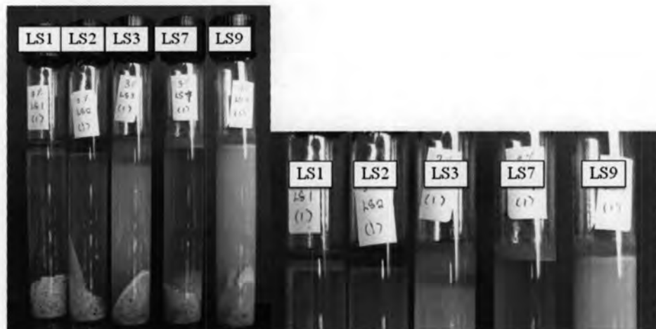
Figure 4.1 Photos of extraction results by surfactant systems of LS series
