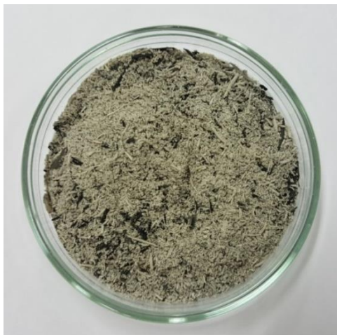
Fig. 18 – Rice hull ash after incomplete combustion
