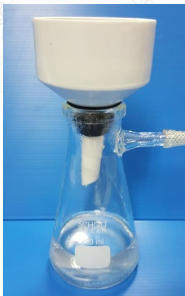
Fig. 20 – The dispersion was filtered through Whatman grade 42 ashless filter paper and then washed with 100 mL of boiling water
