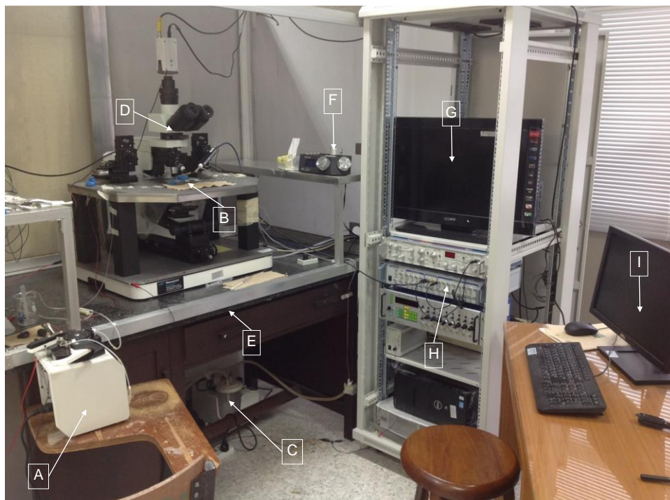
Figure 7. Whole cell patch clamp set up recording; A: Peristaltic pump, B: Culture dish, C: Vacuum pump, D: Up light microscope, E: Anti-vibration isolation table, F: Manipulator, G: LCD monitor, H: Axopatch 200B amplifier, I: pClamp10.2
