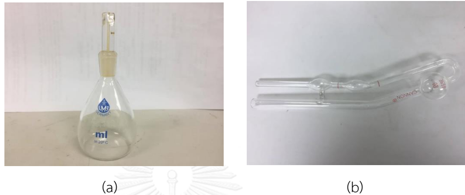
Figure 4.2 Equipment for measuring density and viscosity (a) Pycnometer (b) Cannon-Fenske viscometer
