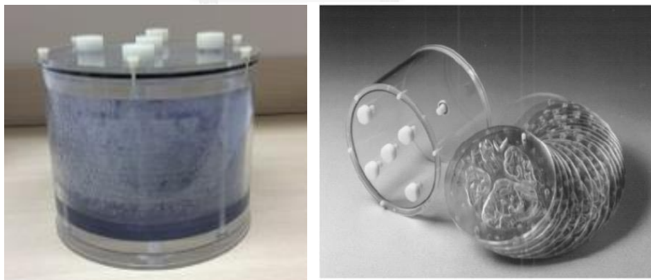
Figure 3.4 Hoffman 3D brain phantom (left) and component of brain slabs inside the phantom (right).
