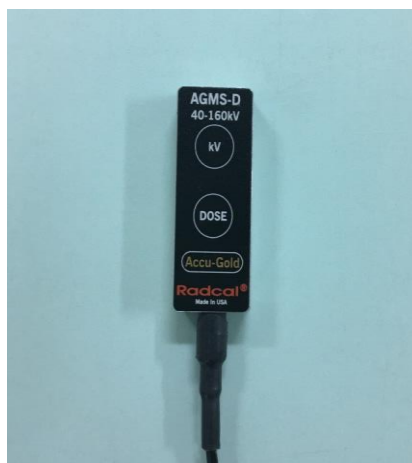
Figure 3.4 The solid state dosimeter dosimeter; Radcal Corporation model ACCU-Gold.
