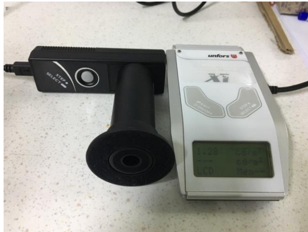
Figure 3.5 The luminance meter manufacturer UNFORS Raysafe model Xi.
