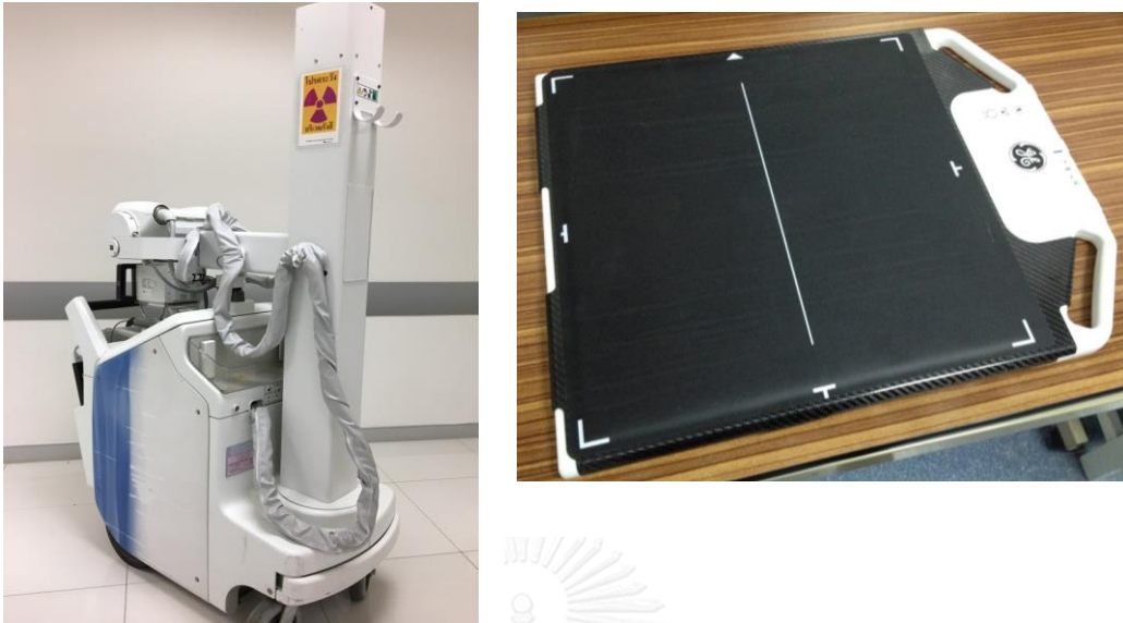
Figure 3.3 Digital mobile x-ray system manufacturer General Electric (GE), model Optima XR220amx and digital receptor with grid.
