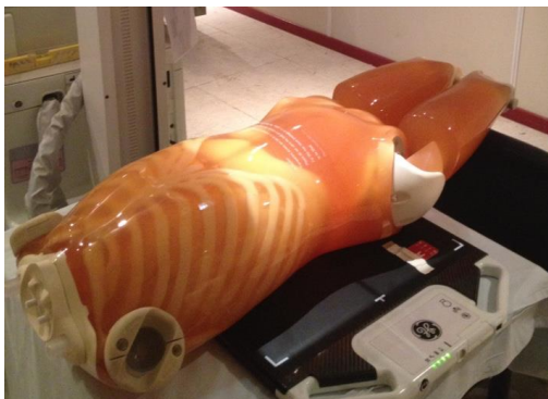
Figure 3.7 The whole-body phantom, KYOTOKAGAKU model PBU-60.
