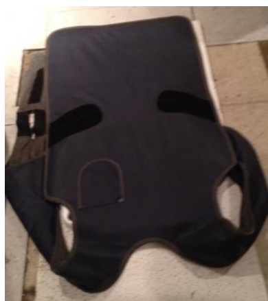
Figure 2. Close the collimators and cover the image receptor with a lead apron.
