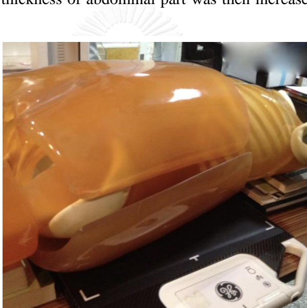
Figure 3.8 The whole-body phantom with buildup layer.
