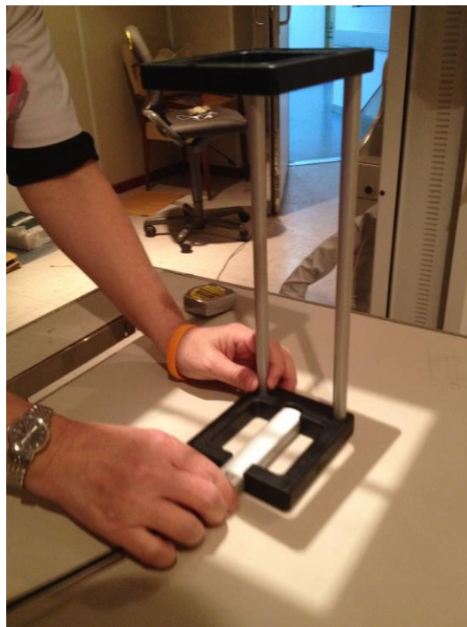
Figure 3. Set up for HVL measurement.
