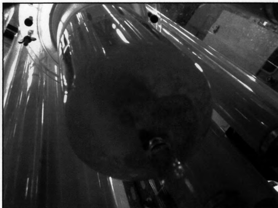
Figure 5.36 Image of the bottom of the bubble column reactor during experiment
