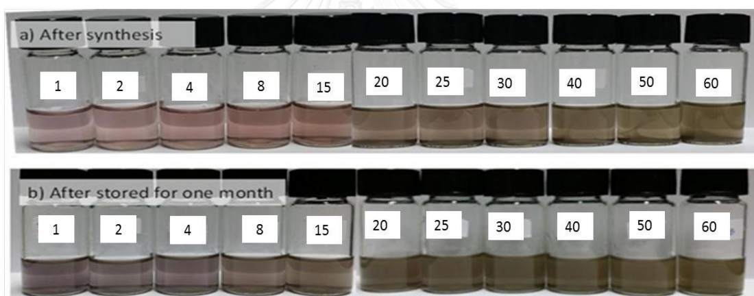
Figure 4.49 Appearances of CS-stabilized silver nanoparticles colloids synthesized using 0.1 mM CS in 1.0 % v/v acetic acid solution at initial pH of 5.0 at various radiation times of 1, 2, 4, 8, 15, 20, 25, 30, 40, 50 and 60 minutes after synthesis and after stored for one month
