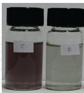
Figure 4.43 Appearances of silver nanoparticle colloids synthesized using initial pH of chitosan at 5.0 (left), and 6.0 (right) after UV radiation for one hour
