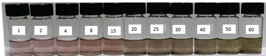
Figure 4.44 Appearances of silver nanoparticles colloids synthesized using 0.1 mM CS in 1.0 % v/v acetic acid solution at initial pH of 5.0 at various radiation times of 1, 2, 4, 8, 15, 20, 25, 30, 40, 50 and 60 minutes
